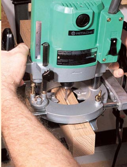
Start the inlay work on the four legs by using a router with an edge guide to rout the 1/4"-wide channels for the inlay.
