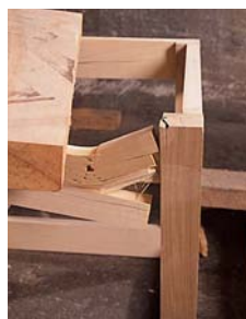
The mortise-and-tenon cube after the first hit.
