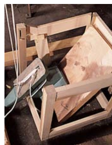
The mortise-and-tenon cube after the second hit.
