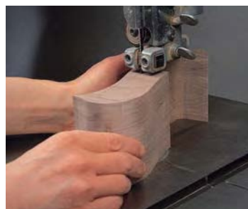
If you take it slowly, a ⅜" blade can achieve sharp curves in the corners when hollowing out the drawers.
