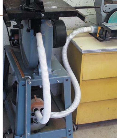
I've placed my shop vacuum under my band saw and next to my sander. A flip of the switch paddle and my dust is under control, no matter which machine I use.
