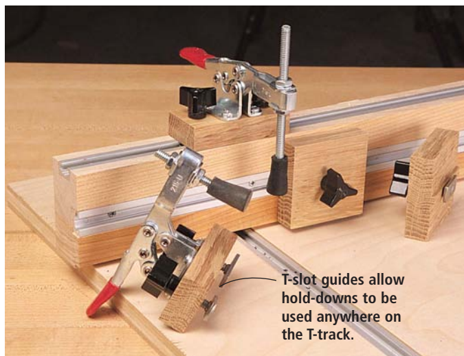
The hold-downs and stops are made from \frac{3}{4} " hardwood. To make the guide that holds the stops squarely on the fence, cut a \frac{1}{16} " x 1\frac{1}{8} " rabbet on both sides of the inside face using your table saw.
