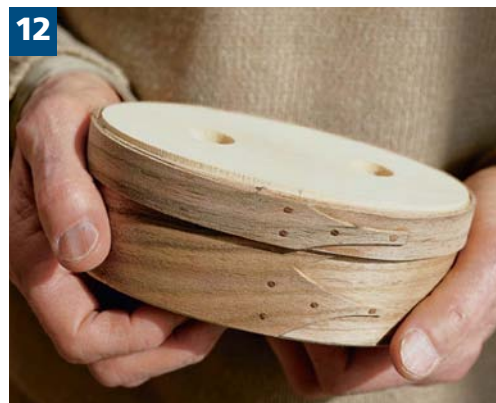
12 The construction of an oval box is half completed when it is set aside to dry for one to two days.
