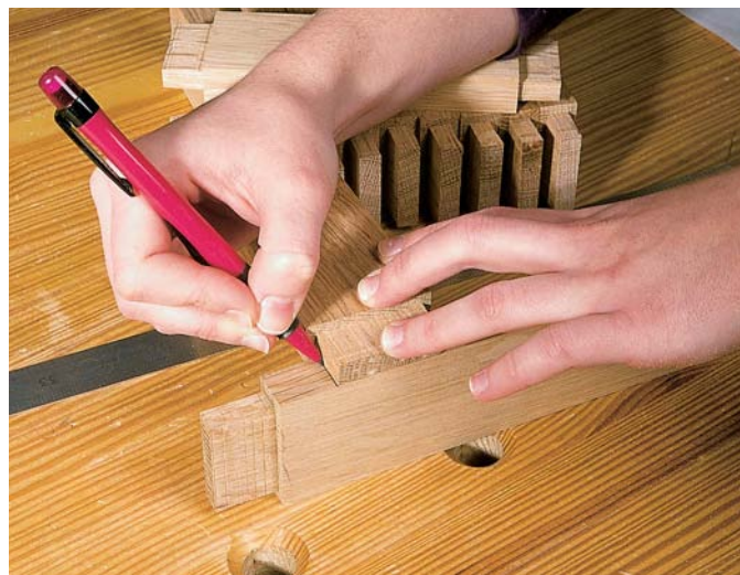
Use the edges of the rails' tenons like rulers to mark the beginning and end of each mortise in the stiles.
