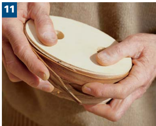
11 The top band is wrapped on the box itself. It will be tacked and then returned to the box for drying. Note that the direction of the fingers match the bottom band fingers.
