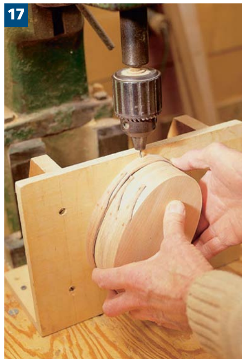
An alternative drilling method makes use of a drill press. The jig, which I call a bookend, creates a vertical drilling station.
