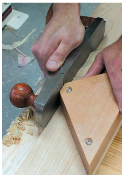
In use, the miter shooting board is used with the plane always pointed toward the stop block.
