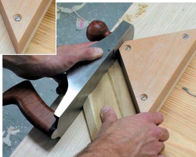
In use, the miter shooting board is used with the plane always pointed toward the stop block.
