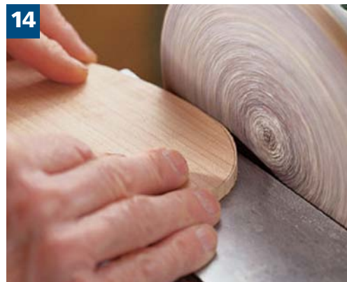
14 The disc sander finishes the edge up to the pattern line. The sander table is elevated to 4^\circ to provide a slight cork effect to this ellipse for a tight fit. To make this adjustment, you may need to file out the slide slot so it no longer stops at 0^\circ , or you can remove the thumb screw and use a small C-clamp.
