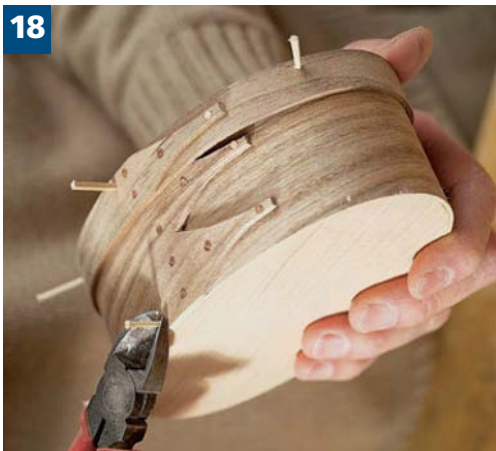
Wood pegs are made from cutting in half the box of World's Fair Brand toothpicks. The tapered end to these match the \frac{5}{64} " hole for a secure fit when tapped in place.
