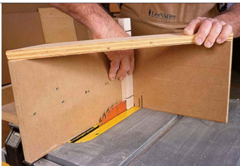
Cut the cheeks using a tenoning jig – this one is shopmade. For the cut, adjust the blade to match the width of the stock. Position the jig and the work so the waste falls to the outside of the blade.
