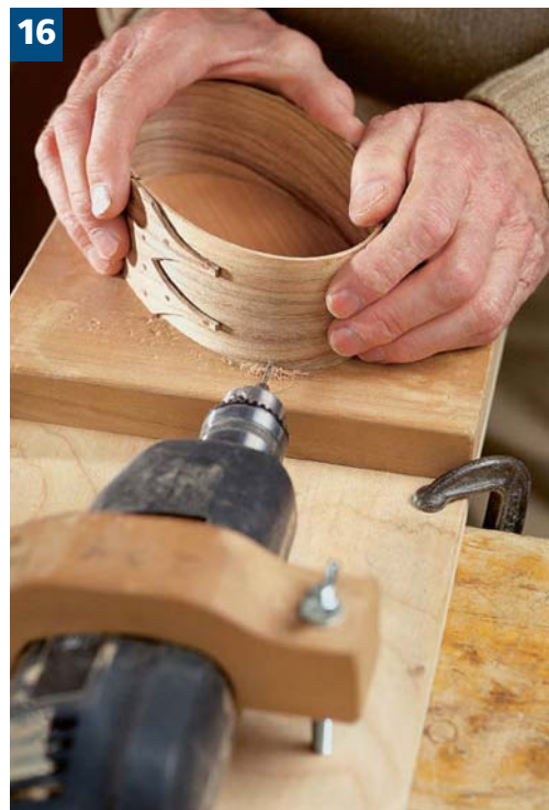
After the oval board is in place and sanded flush, drill the perimeter every 2" to 3" for wood pegs. This drill jig locks a spare drill to a board with a front table the right height to center the hole on the \frac{1}{4} " board inside.
