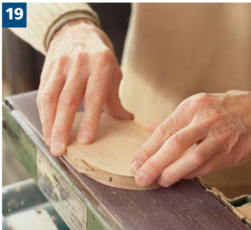
Final sanding is done with a 120-grit belt replacing the 80-grit one used for shaping wood before.
