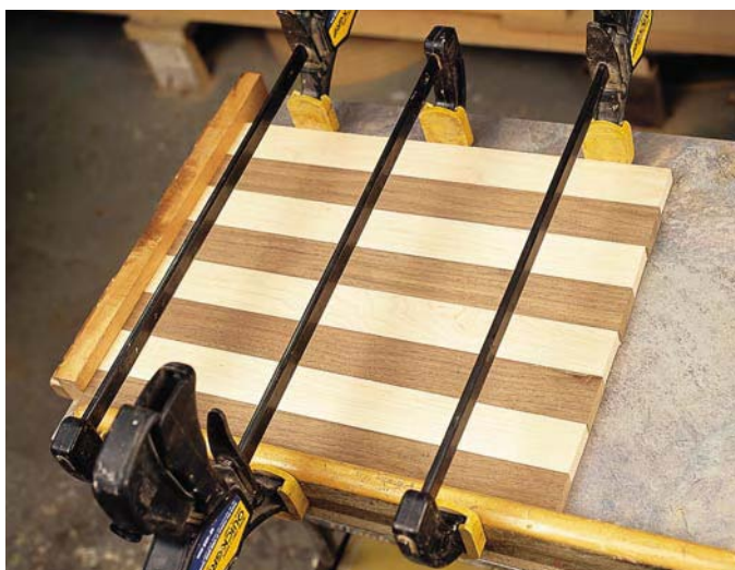
The first step in making a gap-free chessboard top is to glue together eight maple and walnut strips, alternating between the species.
