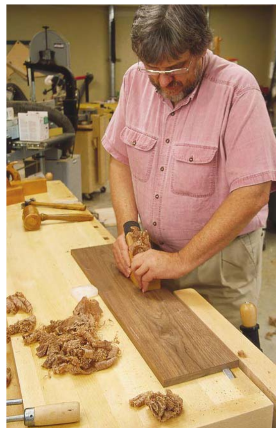
A properly tuned wooden plane is a joy to use. Nearly every surface of traditional 18th-century furniture was shaped or smoothed with a wooden plane.
