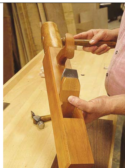
To make a lighter cut, tap the heel of the plane with your mallet and then tap the wedge. Some planes have a “strike button” on the topside of the tool's stock in front of the blade. You also can tap the strike button to reduce the cut.
