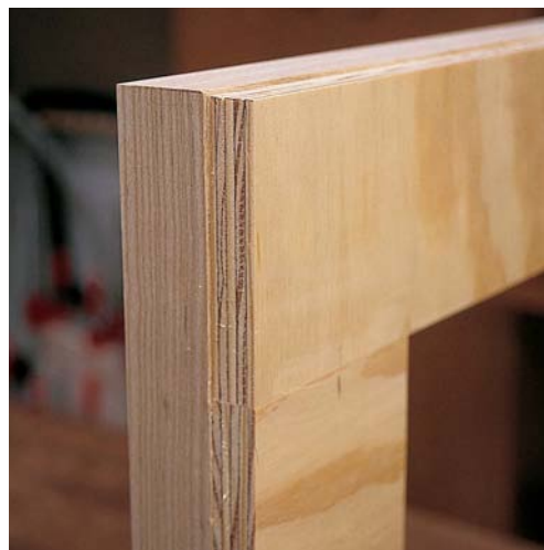
Here you can see the \frac{1}{16} " lip created by the straight moulding when attached to the inner top panel.
