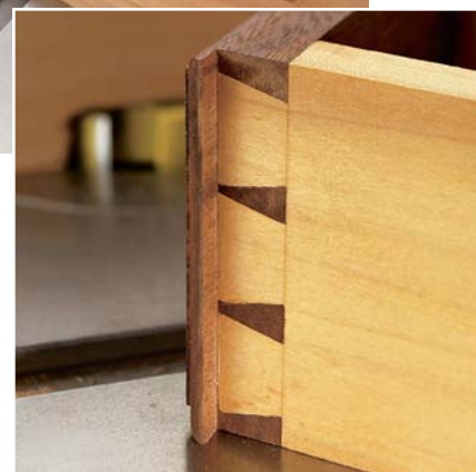
Cutting a lip on the backside of a drawer front is a common shaper operation (above). With this simple fence, the entire drawer front is in contact with the fence throughout the cut, and there's little opportunity for tearout. Lipped drawers are commonly used in conjunction with half-blind dovetails.
