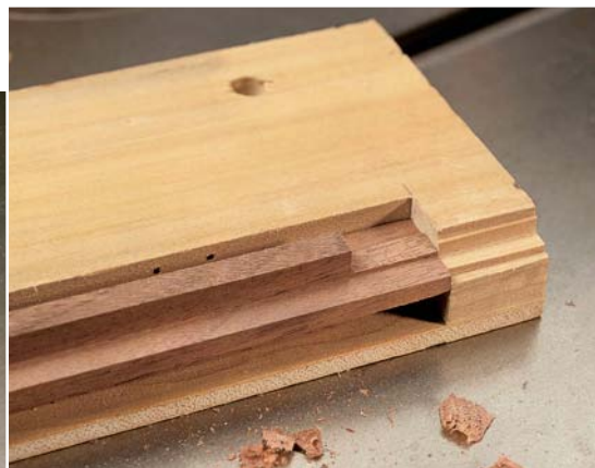
Shaping mullions and muntins on a shaper (or even a router table) can be intimidating. This jig has a notch in the edge that holds your work down and against the fence.
