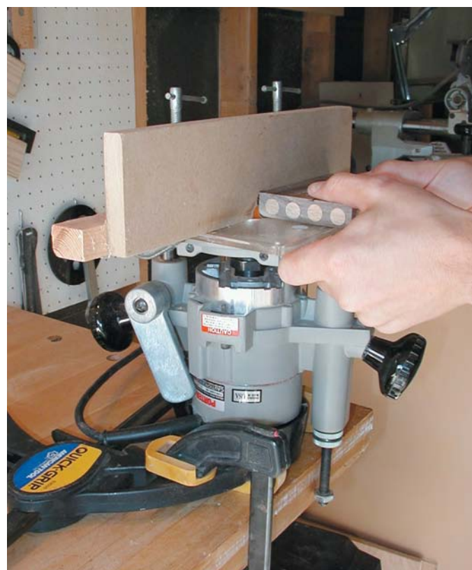
You can make a tiny router table simply by attaching a MDF fence to your router's base. Pivot the fence into the ogee bit until the roundover section pokes through.
