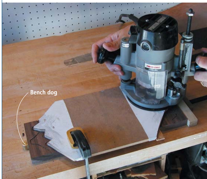
Use double-stick tape and the dogs on your bench to secure the maze block to the routing template.
