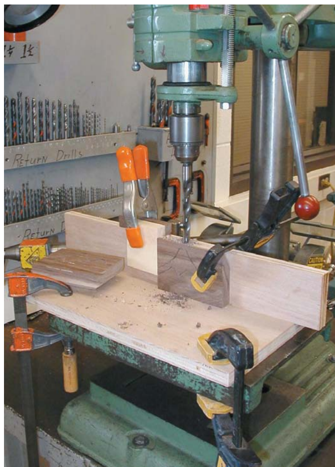
You'll need a full-size drill press to bore the deepest holes in the maze. The machine's "throw" should be at least 2\frac{3}{4} ". Make sure to clamp the block to a fence. If the block moves even a little, the bit might catch and ruin your block. (Remember the extra blocks you cut?) Use a stop block to eliminate errors that come from repetitive measurements.
