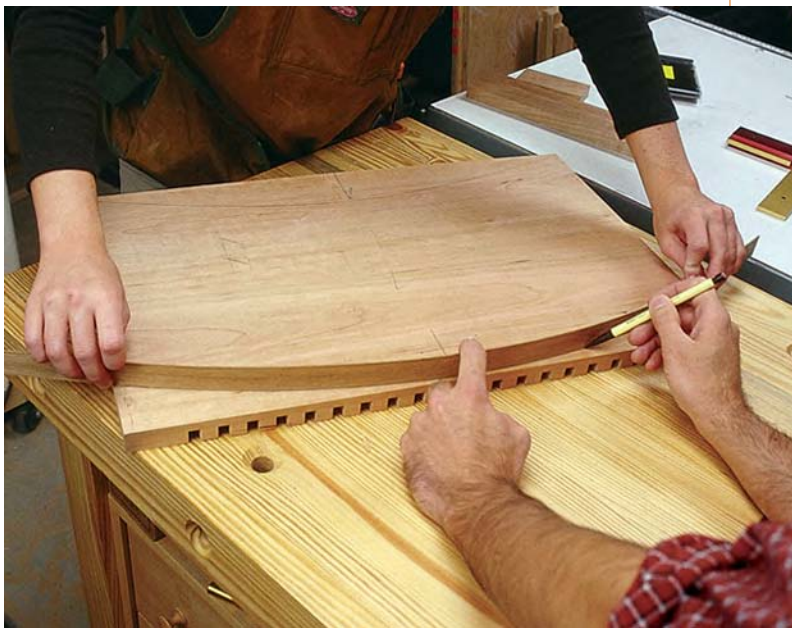
Laying out curves often requires extra brad nails or extra hands. To lay out this curve we marked the center of the panel and then measured 2\frac{1}{2} " down on either end. We then tapped three nails at each mark. One person held a thin piece of wood at each end nail, while the other person held the wood to the center nail and drew the curve.
