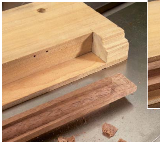
Shaping mullions and muntins on a shaper (or even a router table) can be intimidating. This jig has a notch in the edge that holds your work down and against the fence.
