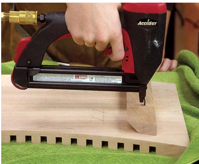
Here you can see I'm attaching the French cleat to the back of the curved wall-hung rack. This cleat, along with another block of wood that's attached further down the piece, will make the rack look like it's floating on the wall once hung.
