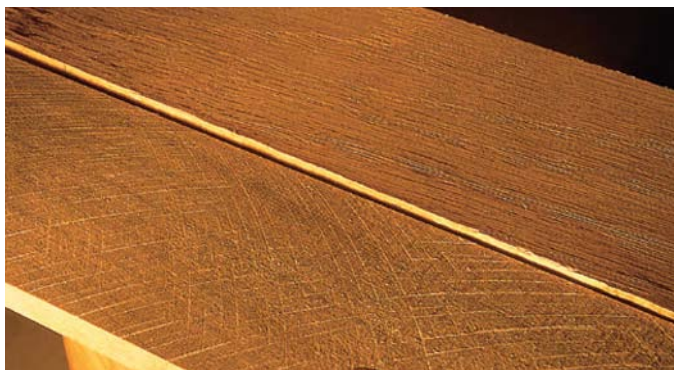
A properly adjusted fence will result in a cut with cross-hatched tooth marks. The board in front was cut with a 24-tooth rip blade. The board in back was cut with a premium-quality 40-tooth blade.
