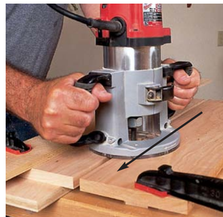
Position the mating board opposite the first, with a gap just smaller than the diameter of the bit between the two workpieces. The feed direction when routing the second edge is left-to-right.
