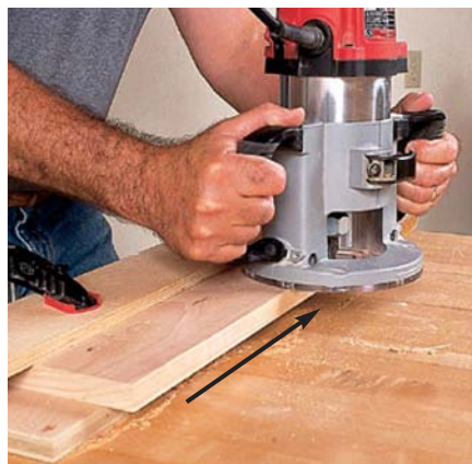
Route the first half of an edge joint by guiding the router along a fence clamped atop the workpiece. The feed direction here is right-to-left (moving away from the camera).
