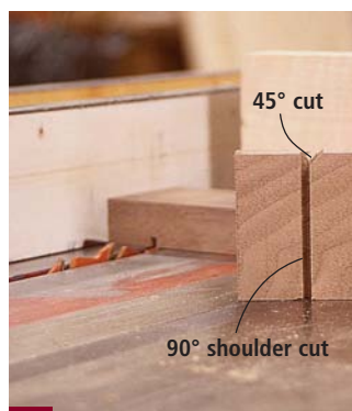
8 Create the same 45° cut in each rail at the required location, then reset the blade to 90° and complete the cut that defines the shoulders.
