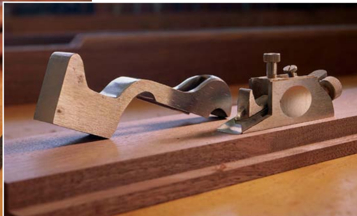
Some shoulder planes, such as the Stanley #92 shown here, feature a removable front piece, which transforms the tool into a chisel plane.
