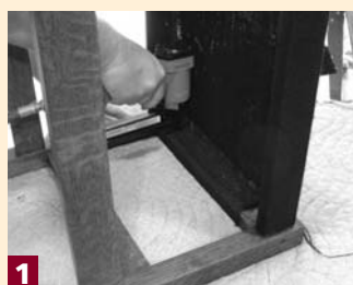
1 Start by mitering the corners of the muslin around the legs and tacking the edges to the inside of the rails, tightening the material as you go.
