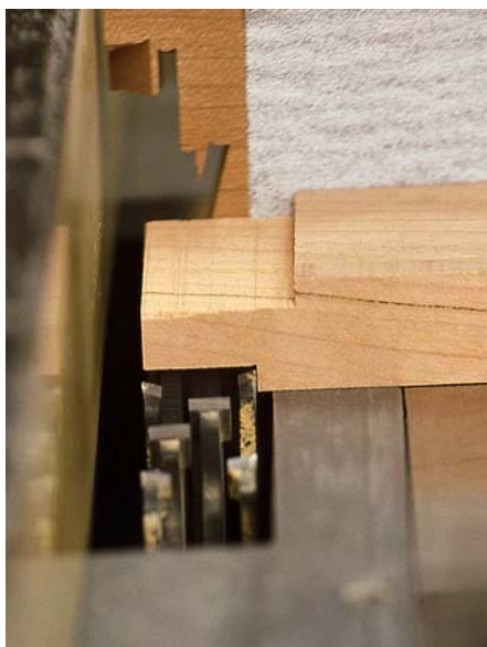
When making tenons with a dado stack in your table saw, the first pass should remove the bulk of the material. Keep firm downward pressure on your work, which will give you more accurate cuts.
