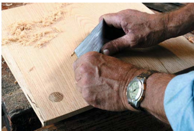
The simplest and most useful of tools, a properly tuned card scraper is the tool to use to prepare a surface for finishing at all stages of the project.
