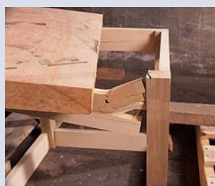
3) The mortise-and-tenon cube held together after the first hit.
