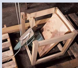
4) The mortise-and-tenon cube collapsed after the second hit.
