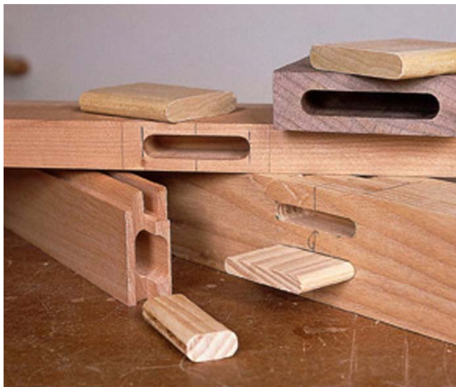
A plunge router, an edge guide and a shop-made jig are the foundation for loose-tenon joinery.
