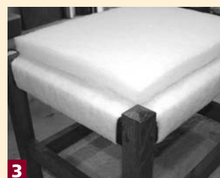
3 A layer of 2" foam will add cushion. The piece should be cut to fit just inside the rails and will lay in place on the first batting layer.
