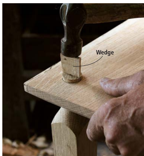
The wedges lock the legs in place and tighten up the fit between the tenon and its mortise.
