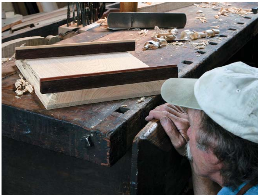
Winding sticks are truth-tellers. They find the bow or twist in any board. Sight down one and compare it to the other to find twisting and cupping. The different colored edges make it easy to see both sticks.
