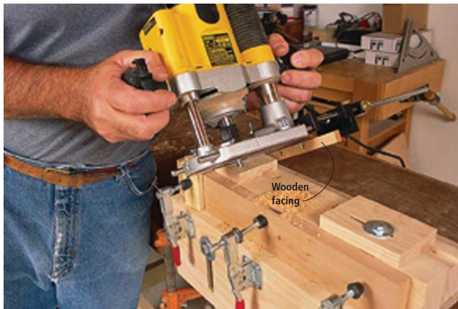
The wooden facing on the edge guide drops into the channel at the back of the jig, allowing you to move the router back and forth without worrying if it will wander off course. The stops control the router's travel, ensuring the mortise will be the correct length.
