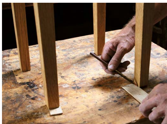
This is an old chairmakers' trick. With the table on a perfectly level surface, you can wedge the legs to make the tabletop sit flat. Then use a spacer that fits under the shortest leg to mark how much you should trim off the other three.
