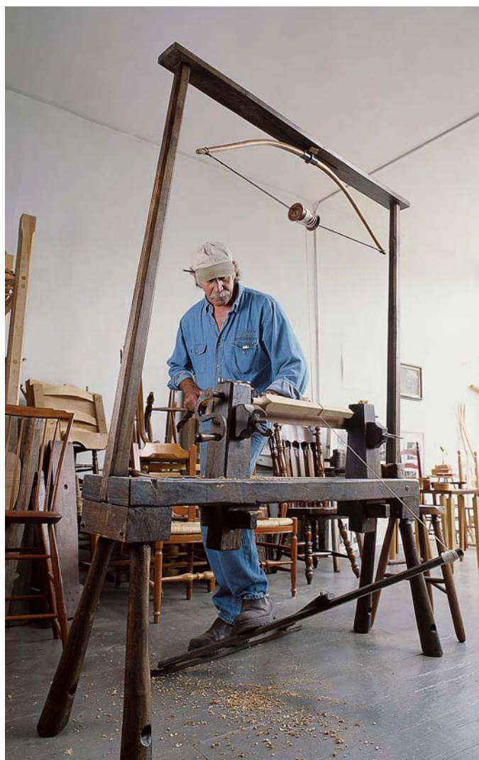
Using a pole lathe is a bit different than using a motorized one. The work rotates toward you on the downstroke and away from you on the upstroke. You cut only on the downstroke. It takes a bit of practice, but you can get used to it.
