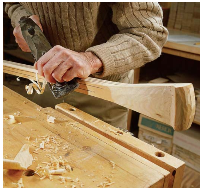
The shaft is planed into an octagon following guide lines.
