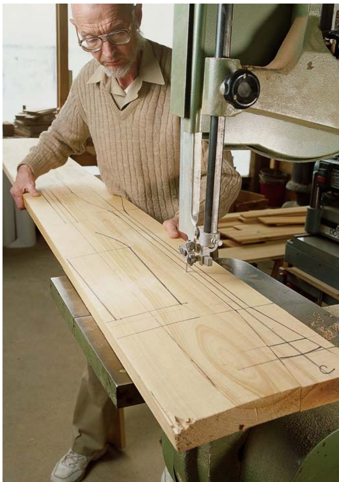
After planing the plank to 1\frac{1}{4} " thick, band saw the paddle blank to shape.
