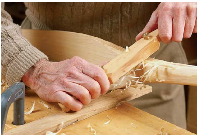
The spokeshave (I'm using a wooden one here) is used to smooth the transition between blade, shaft and handle. It works pulling or pushing to follow the direction of the grain.
