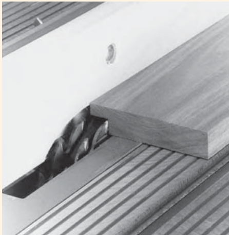
A sacrificial fence attached to your rip fence allows you to accurately use part of a dado set for rabbeting without harming your rip fence. The blade should be run up into the fence while it's securely locked in place to the tabletop. Make sure the blade clears your rip fence.
