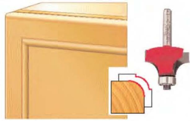
Flat panel with moulded edge and applied moulding 3/8" beading bit, #34-114
