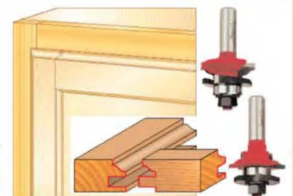
Frame and flat panel 3/8" door lip bit, #99-001 (not shown) Matched rail & stile bit set - ogee, #99-261
