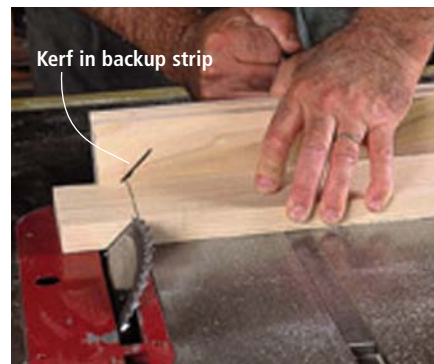
A backup strip attached to the miter gauge aids when you are trying to locate the bevel cut. Align your layout line with the kerf in the strip.
