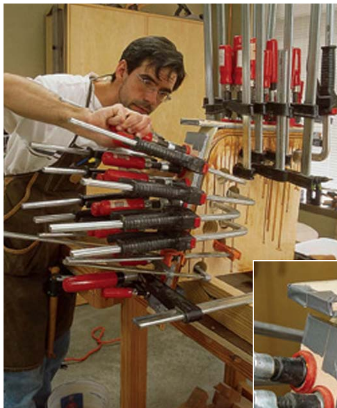
Turn off the radio, hold your calls and don't stop to chat during this part of the project. Speed and accuracy make a good lamination. This glue can set up fast.
