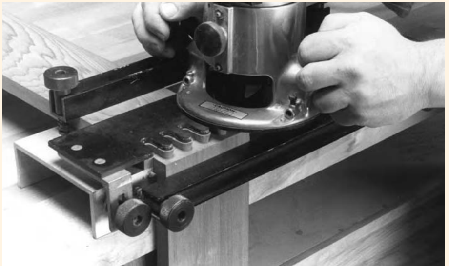
On half-blind dovetails (above), the joint is hidden from view on one side. This makes it ideal for the fronts of drawers and other applications where you don't want to see the joinery. Through dovetails (right) are visible from both sides and are often used for decoration, as well as joining.
