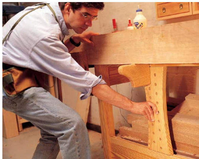
While flattening the top is the most important upgrade, a close second is the sliding deadman. This clever bit of engineering will allow you to immobilize doors easily.
