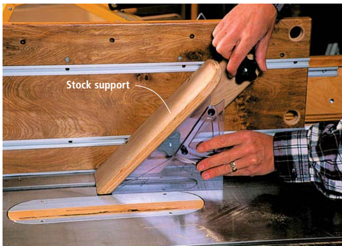
Set up the fixture to cut the feather splines. A drafting triangle set between the underside of the stock support (attached to the sliding rip fence fixture) and the saw table makes quick work of securing the first support at a precise 45° angle.
