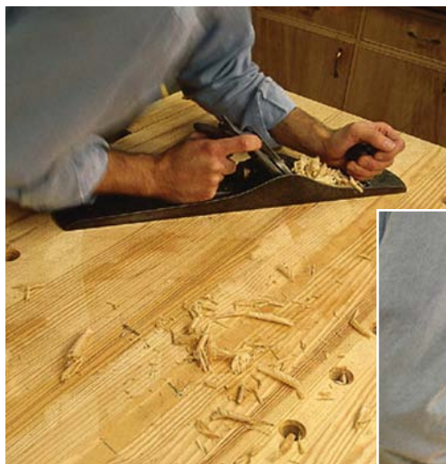
A No. 7 jointer plane's key asset is its length. Because of its length, the plane rides over the low spots and shears the high spots. Begin by working diagonally; don't worry about tear-out (above). When the top is flat from your diagonal passes, plane directly with the grain (right).
