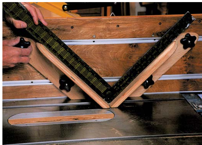
Use a 24" framing square, such as the one shown above, to set the second support square to the first. To see this operation in action, check out page 31 of our December 2003 issue or go to "Magazine Extras" online at popwood.com .
