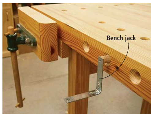
This simple bench jack excels at clamping boards that are 8" wide or narrower. Like the leg jack, this is a quick upgrade.
