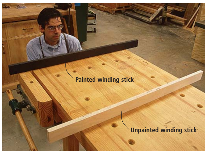
Winding sticks are the key to making sure a benchtop or tabletop is indeed flat. Check the top by moving the light-colored stick to different positions across the length of the bench and comparing the top edge of each stick.
