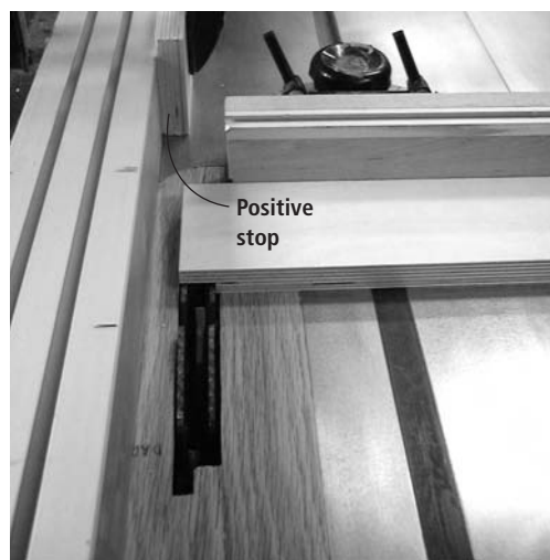
I cut the rabbets with my dado stack and a block of wood clamped to the fence to serve as a positive stop to gauge the rabbet width. It's safer than against the fence.
