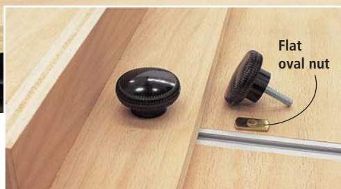
Attach the plywood table, with the tracks already installed, to the adjustable uprights with screws. Secure the fence to the T-tracks using knobs with a threaded shaft and flat oval nuts (right).
