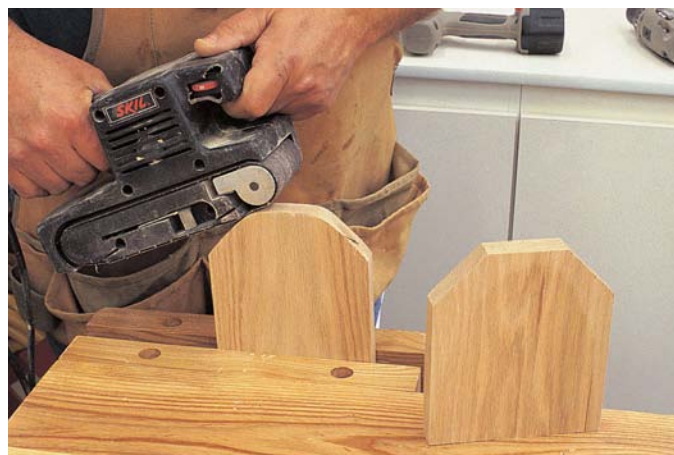
Adjustable uprights for your table also are made with hardwood and shaped to allow the table to pivot.
