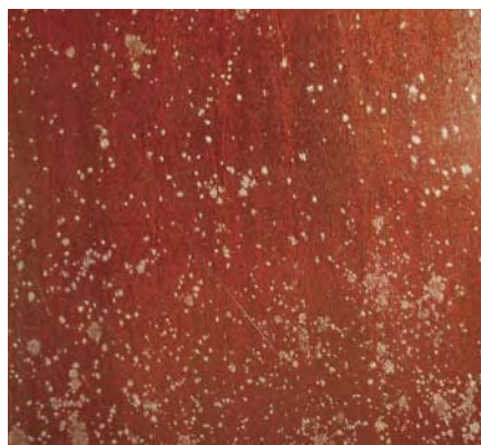
Mildew spores can be killed (to stop further growth) by washing the surface with half-and-half household bleach and water. Dry the surface quickly so the water doesn't damage the finish.
