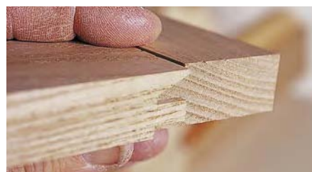
The pieces should come together flush on their faces (left), not offset (right).
