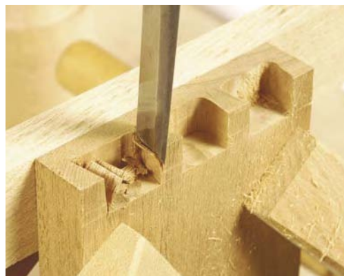
Begin paring away the waste on the sides of the pins. Take small bites. Finish each pin by placing the edge of the chisel right in the knife line and tapping lightly with a mallet.
