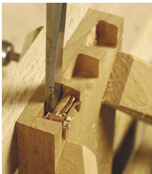
When the sides of the pins have been pared to the line, work on the front of the joint. Make sure the front edge and the sides of the pins are square, not sloped, so the joint will go together without splitting the drawer front.
