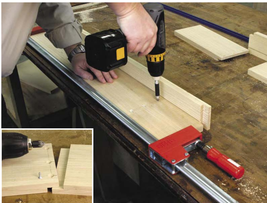
Accurately screwing the mating half-lap pieces together requires clamping the pieces together. Countersunk pilot holes and flathead screws complete the assembly.
