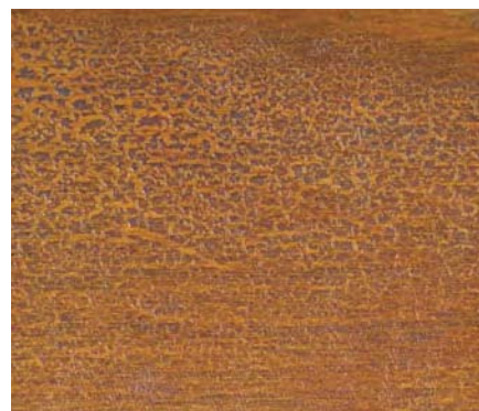
Finishes that have softened and become wrinkled (and also dirty) because of extended contact with acids contained in body oils and sweat (as shown above) usually have to be stripped and replaced with a new finish.
