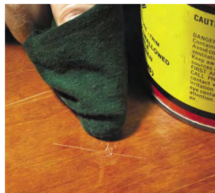
If a liquid makes the scratch too dark, apply some clear paste wax.
