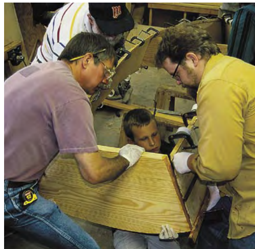
From left to right, Hott, Merlin, Lars and Eisenlord wrestle the assembly of the sides, stem and transom into shape with a temporary spreader to hold the shape of the hull. As you can see, it takes all hands on deck to pull these parts together.
