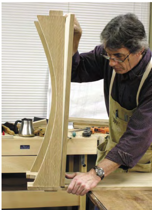
With the two bottom rails in place, I spread glue on the top edges of the rails and in the dado before tipping the bottom in to place.
