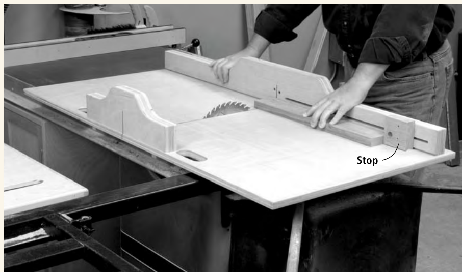
A two-sided miter sled allows equal support on either side of the blade and also functions as a partial blade guard. While stops can also be added into this design (as shown) it doesn't easily allow for adjustable miter cuts.
