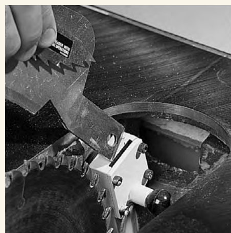
An aftermarket splitter/pawl assembly is shown in position (left) and being easily removed (right), without the use of tools. The splitter keeps a cut board from pinching the blade, while the pawls reduce kickback. The two parts work together to ensure your safety.
