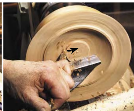
Note the position of the tool as I begin the cut. To keep the bevel rubbing while cutting the side of the bowl, the handle must be held far to the right and must swing around to the left as you cut to the bottom or center of the bowl.
