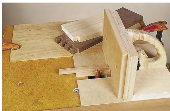
On the router table, I use a small version of the jig. My tables don't have miter-gauge slots, so I align the jig with the selected bit in the slot in the jig base. Then I set a thin plywood strip against either edge of the jig and clamp them to the tabletop.
