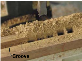
The mortiser is set with the chisel flush with the panel groove. Plunge the bit and chisel to make distinct holes, then come back and clean up the waste in between.
