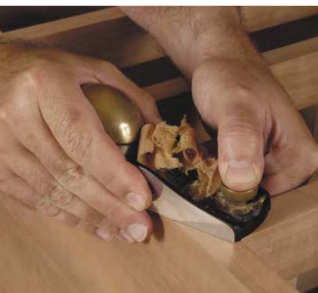
A standard-angle block plane with a 55° cutting angle is useful for leveling the joints. This high cutting angle reduces tear-out in some tricky woods.
