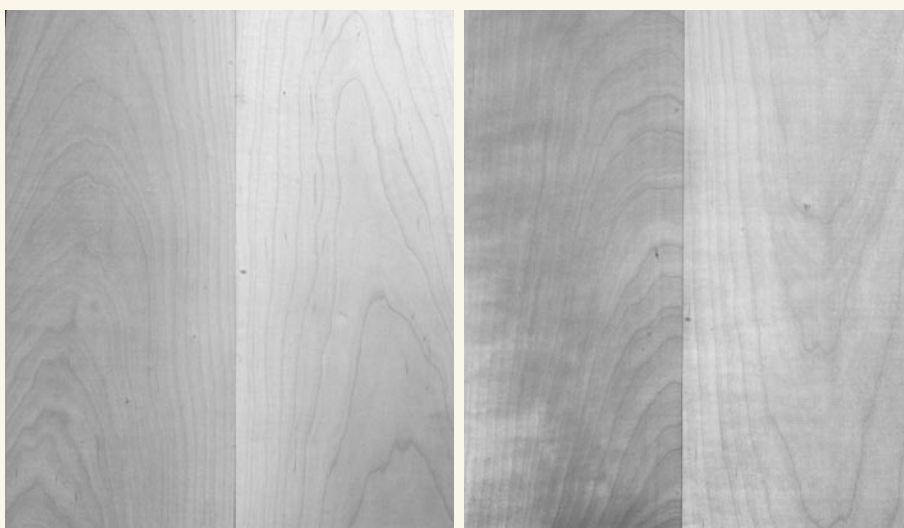
Shown here are two boards arranged to give an example of a good, solid-wood grain match (left) and an example of a bad grain match (right). Even though the boards aren't exactly the same shade, by matching two sections that are long grain, the boards on the left look balanced. The boards on the right have an interrupted cathedral and the cathedral figure on the far right board is pointing the wrong direction.
