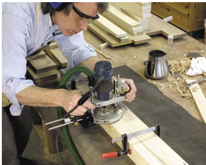
A group of stiles for the web frame is clamped together to lay out the joints. Leaving the stack clamped together provides a stable base for the router used to cut the mortises.
