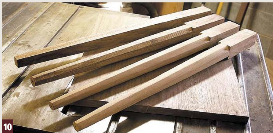
10 The two legs in front have been finished. The one immediately behind them has had the second set of facets sawn but not planed. The leg at the rear has had only the first set of facets sawn and planed, although the shoulders for the second set have been defined by a backsaw cut.
