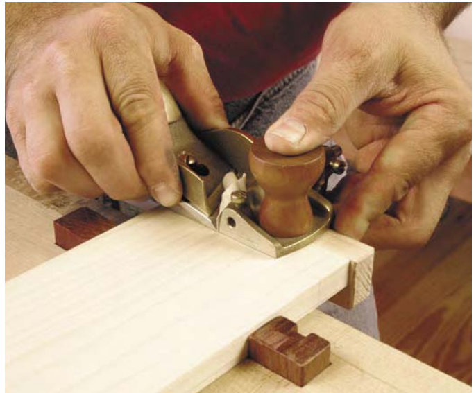
Cutting a shallow rabbet on the tail board will help you mark your pin board later. The pin board will drop into the rabbet, which will increase your speed and accuracy.
