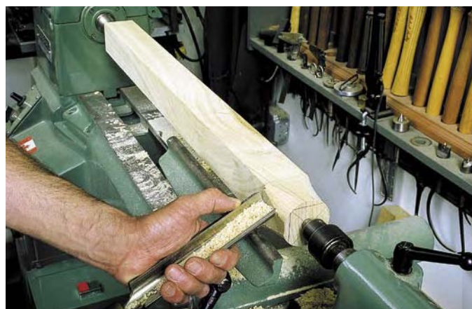
First the blank is mounted on "axis B" and the foot is made round with a roughing gouge.
