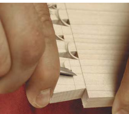
Chamfering the inside edges of your tails will make your joint assemble more easily. I use a chisel.
