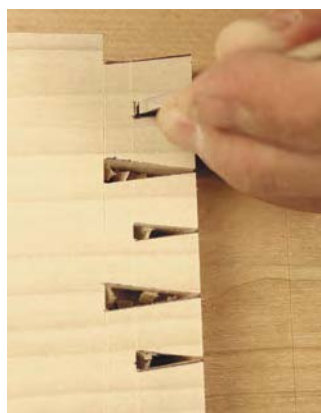
A small bevel-edge chisel allows me to remove any additional waste between the tails.
