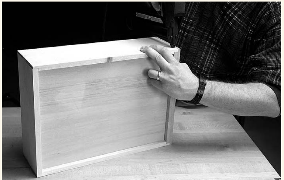
Two rabbeted joints are shown on this drawer. Simple in the back, with the rabbet cut only in the sides, while the front joint incorporates a dual-rabbet joint. In either case a nail (with glue, of course) will make the joint much stronger.
