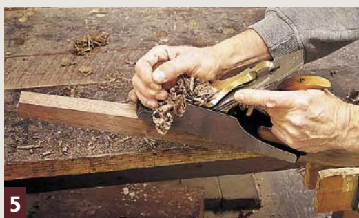
5 After the first four tapers have been cut, fix the untapered apron section of the leg blank in your vise. Then plane away the saw marks on the taper.
