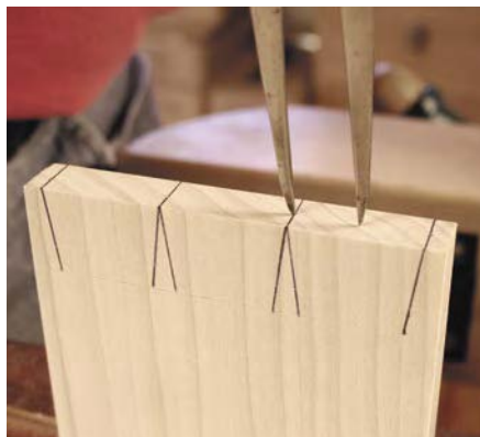
Use your dividers to step off three tails as shown (and marked in ink). Then reset your dividers to divide those tails in half for the houndstooth.
