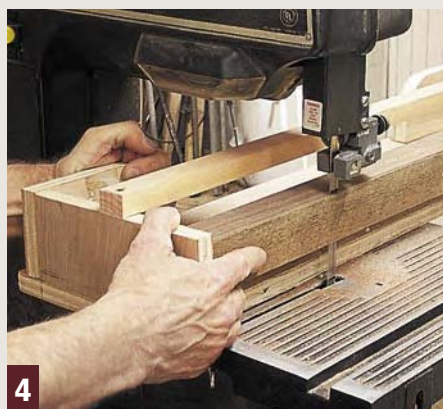
4 Cut those first four tapers by passing the cradle past the band saw blade.
