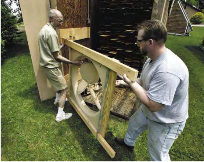
Before loading, the end of the kiln is opened by a hinged door panel and unscrewing a 4'-wide main panel. The 30" fan is being removed to give access.
