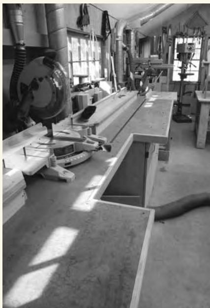
A power miter saw centered on a bench against a wall can cut be used to cut long pieces of stock into more manageable pieces. By locating the saw near the entry door and storage racks, you won't have to maneuver long pieces of wood through the shop.
