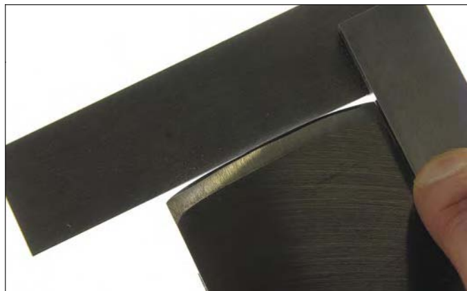
A silhouette of the shape of my fore plane's cambered iron. It's an 8" radius, which allows me to take an almost \frac{1}{16} "-thick shaving in softwood.
