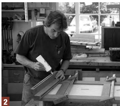
2 The back assembly (with pre-finished panels) is already in the clamps, except for the corners. They're the final addition to the back assembly.
