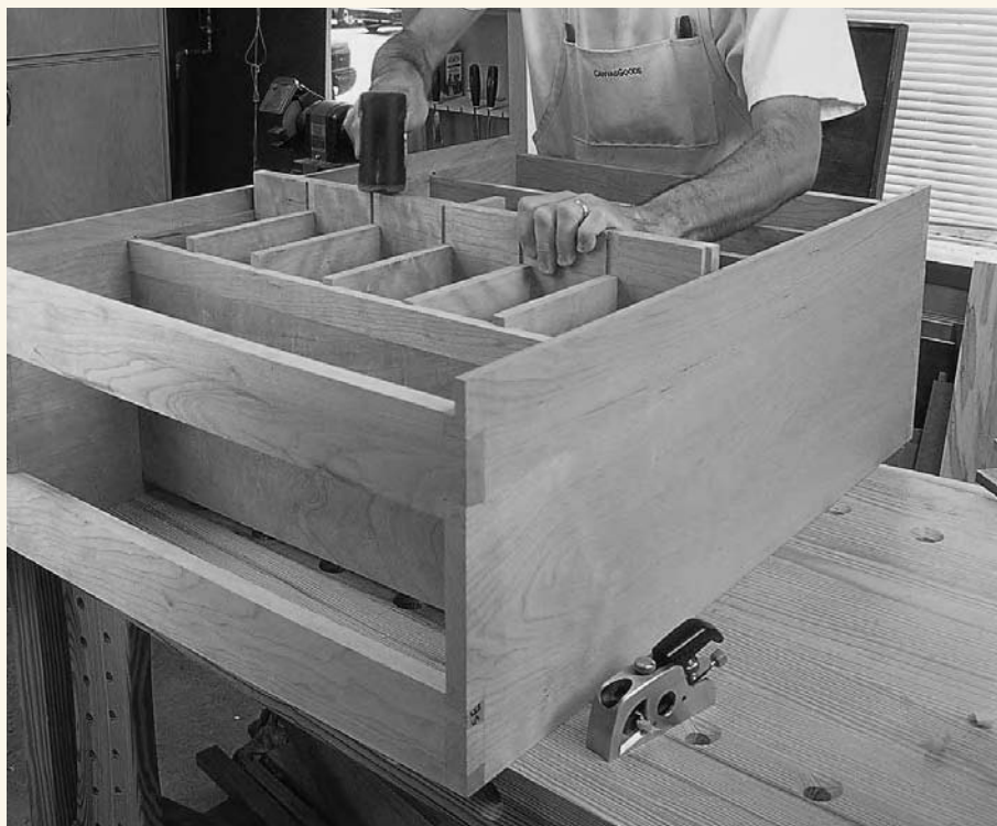
Fitting each of the interior dividers in this case can take a while, but it's well worth the effort. The plane shown in the right corner of the photo is the correct tool. A shoulder or rabbet plane allows you to fine-tune joinery prior to assembly for a less stressful experience. Once the glue is on the pieces, the mallet is used to tap everything into place.
