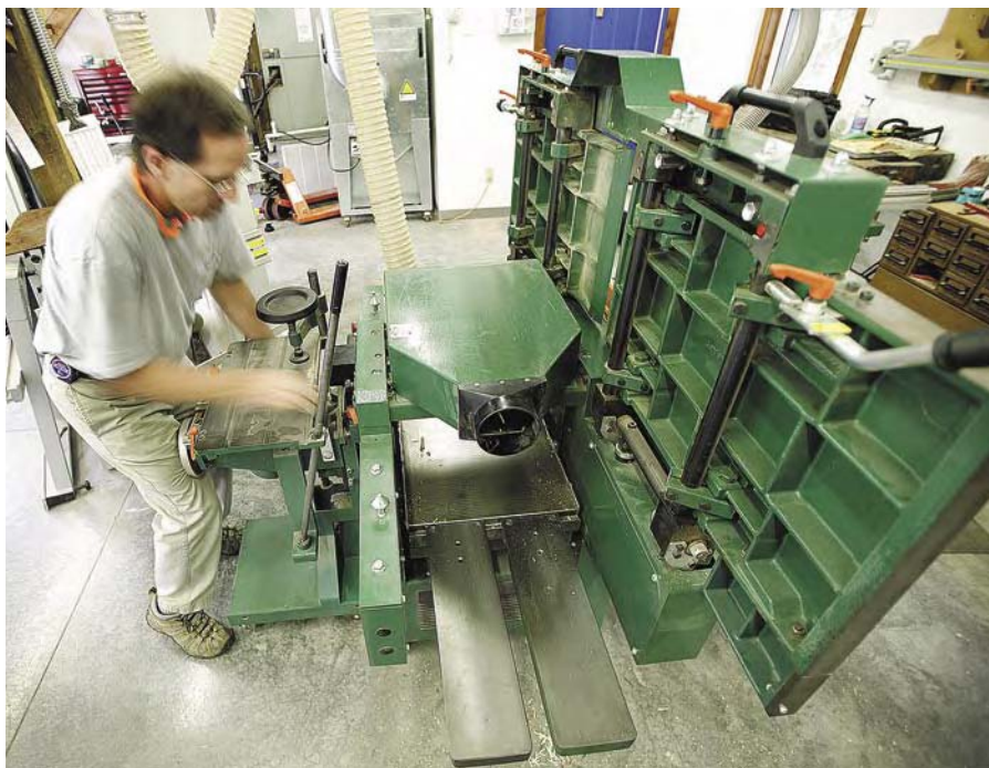
Mehler chose this Felder combo machine (jointer, mortiser, sliding table saw and shaper) because he insists that it incorporates superior safety features.
