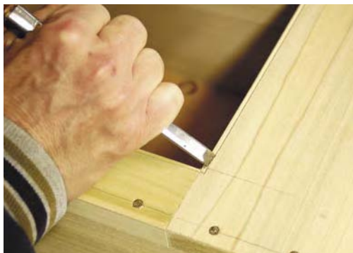
The junction of the horizontal and vertical beads must be completed with a little paring chisel work.
