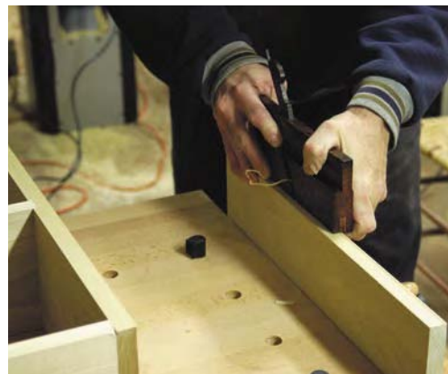
Although the bead on the Shaker original was likely made with a scratch stock (because there is evidence of this tool everywhere at Pleasant Hill), I chose an \frac{1}{8} " side-bead plane.
