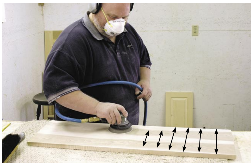
Pattern 2: Now work across the grain. Overlap your strokes and work all along the grain, then back again.
