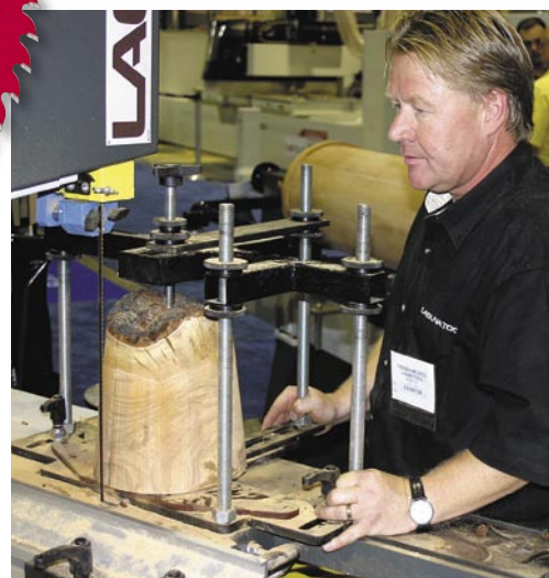
Torben Helshoj demonstrates the Laguna Tools Circle Master accessory, which allows you to quickly turn logs into round bowl blanks.
