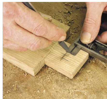
After fitting the through tenon, the location of the second mortise is laid out, keeping the back of the hole just behind the face of the rail.
