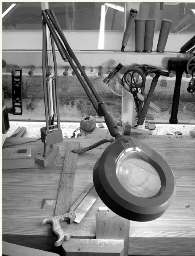
This articulated lamp fits into dog holes on Editor Chris Schwarz’s bench and can be moved as necessary for detail work.
