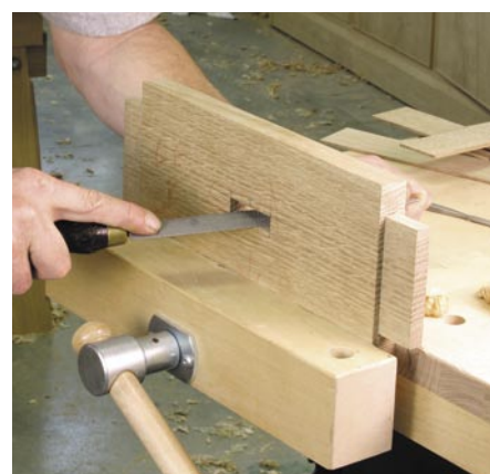
After squaring the corners of the mortise with a chisel, I use a rasp to finish smoothing the inside of the angled joint.
