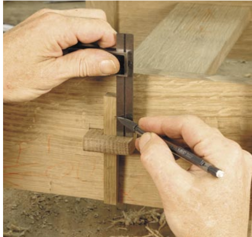
As the tenon key is fit, the length above and below the through tenon changes. I leave the key long and mark the length once I have a good fit.
