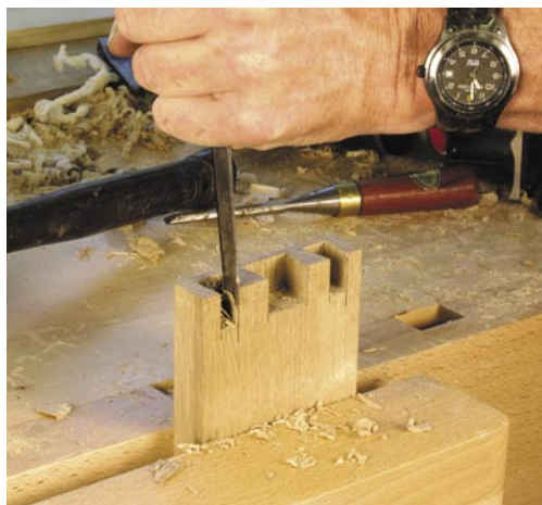
After routing most of the waste, I use a chisel to pare the pins down the rest of the way. The router quickly establishes a consistent depth.
