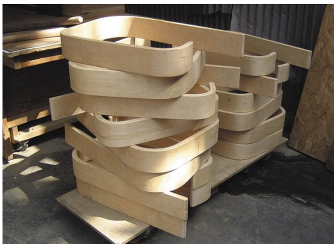
Modern sculpture? Yes and no. A pallet of C-Chair bent lamination arms/legs wait patiently for assembly, finish and upholstery.
