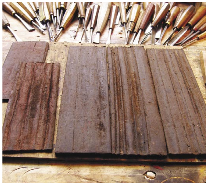
Thick leather soaked in oil is used for a strop. Grooves cut in the leather give the strop the exact shape of the tool.
