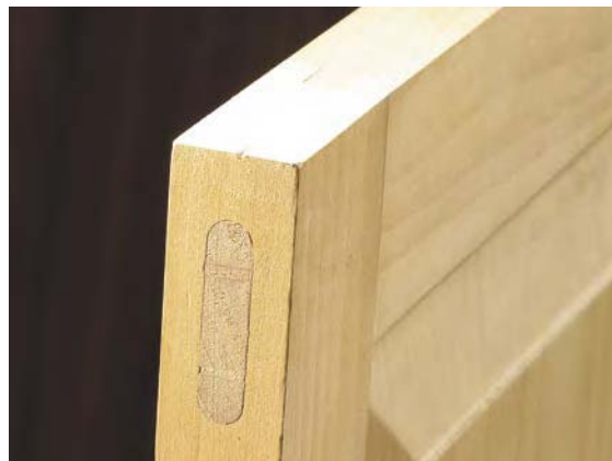
The router leaves mortises with rounded ends. Square them off with a chisel, or round the ends of the tenons to match.
