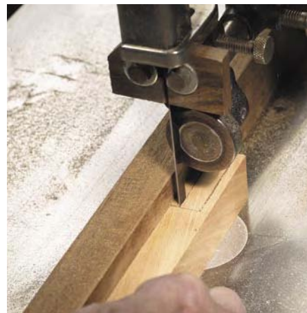
The fence on the band saw lets you make long straight cuts on the cheeks of the tenons.
