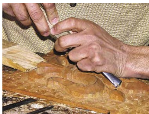
The bevel on the inside of the tool creates another shoulder, allowing the tool to cut both concave and convex shapes.
