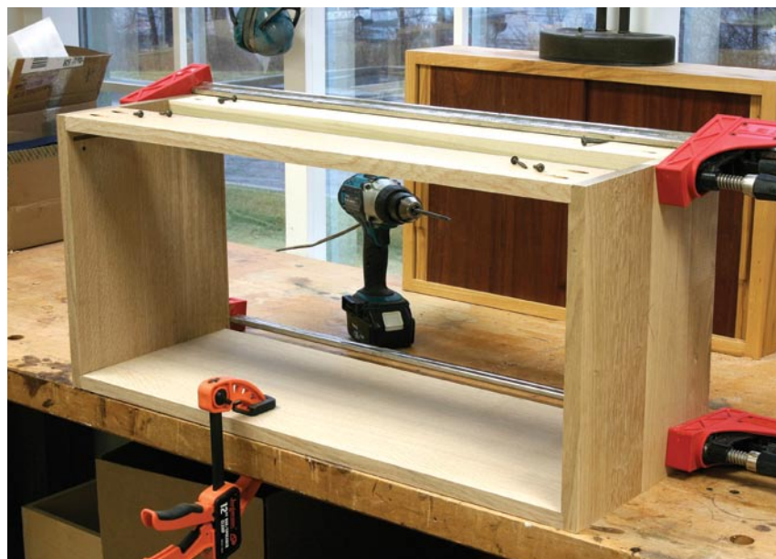
Assembling the boxes is a matter of 14 pocket screws. Clamping the box ensures that it will be square. The opening in the top is for the adjoining catch rail on a second unit.
