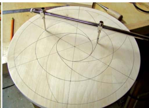
The layouts for both a four-jaw and a six-jaw chuck. (You could use a trammel for both layouts.)
