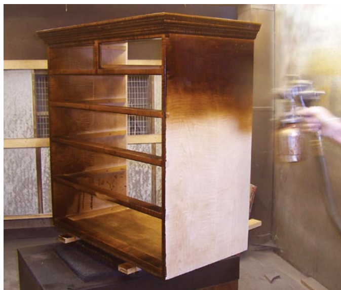
Any case can be stained with a high-volume low-pressure (HVLP) system. Flood the surface when applying stain. Let the stain soak into the wood in order to get the best results.
