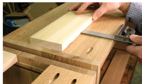
The catch rail is fastened to the box bottom. It is important to properly align the piece to fit the other units.
