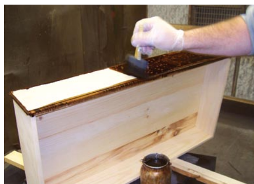
The most effective way to apply the stain to a drawer front without getting the interior of the drawer covered is to use a foam brush.
