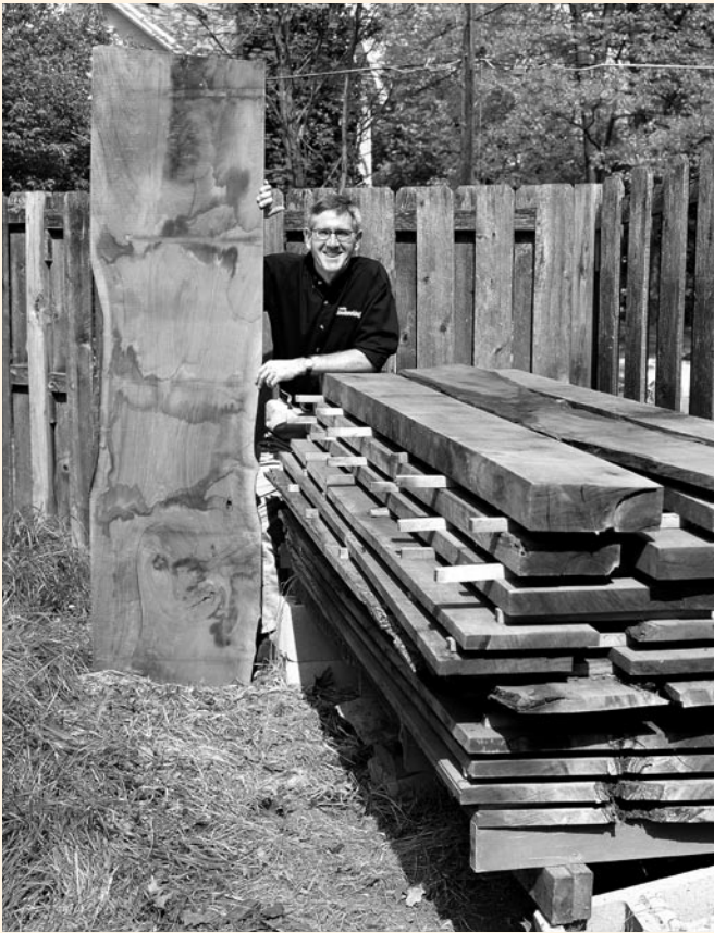
Careful stacking will help preserve these walnut boards for Popular Woodworking Publisher Steve Shanesy. The wood pile should start on a flat base elevated off the ground.
