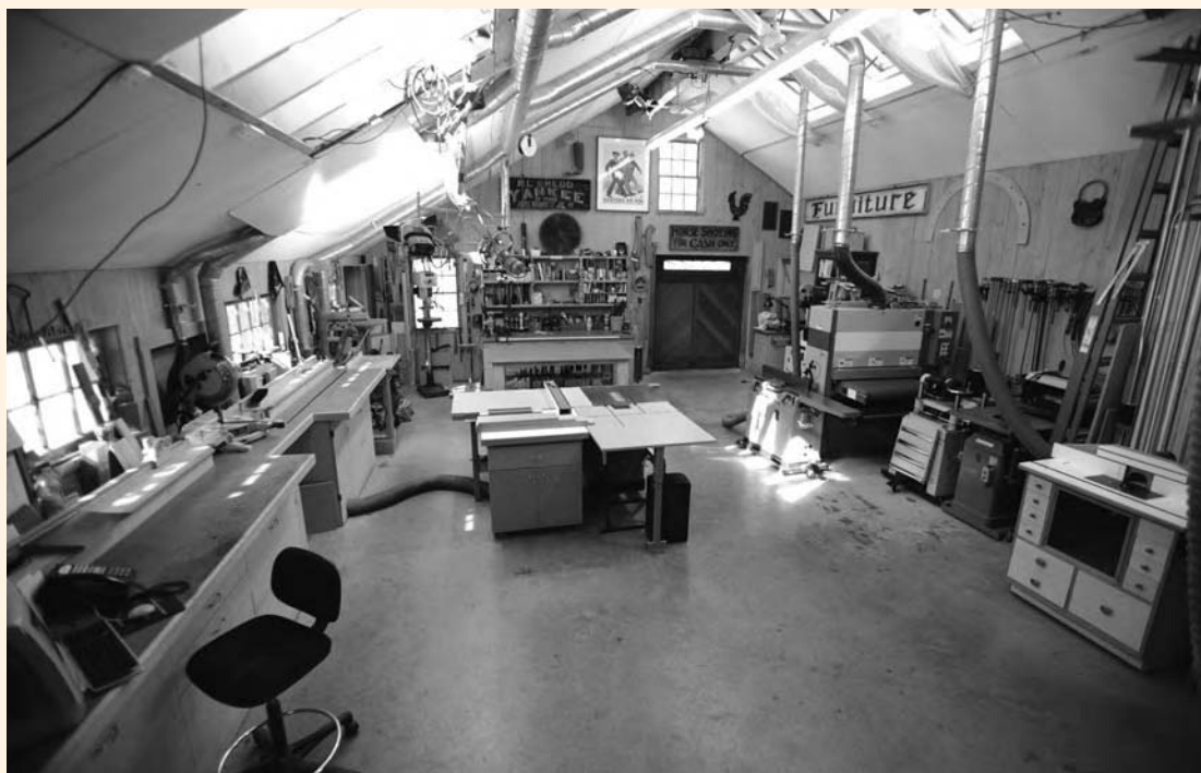
Norm Abram's workshop includes a central dust-collection system that keeps the shop both cleaner and a lot safer. No matter what the equipment, dust collection is important in any sized shop.
