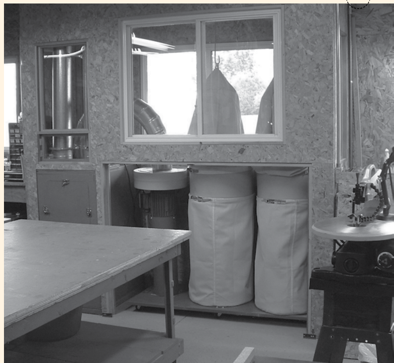
George Jaeger put his dust collection system in a bump-out along one wall of his Kentucky workshop. Windows let in the light and a removable panel gives him access for cleaning.
