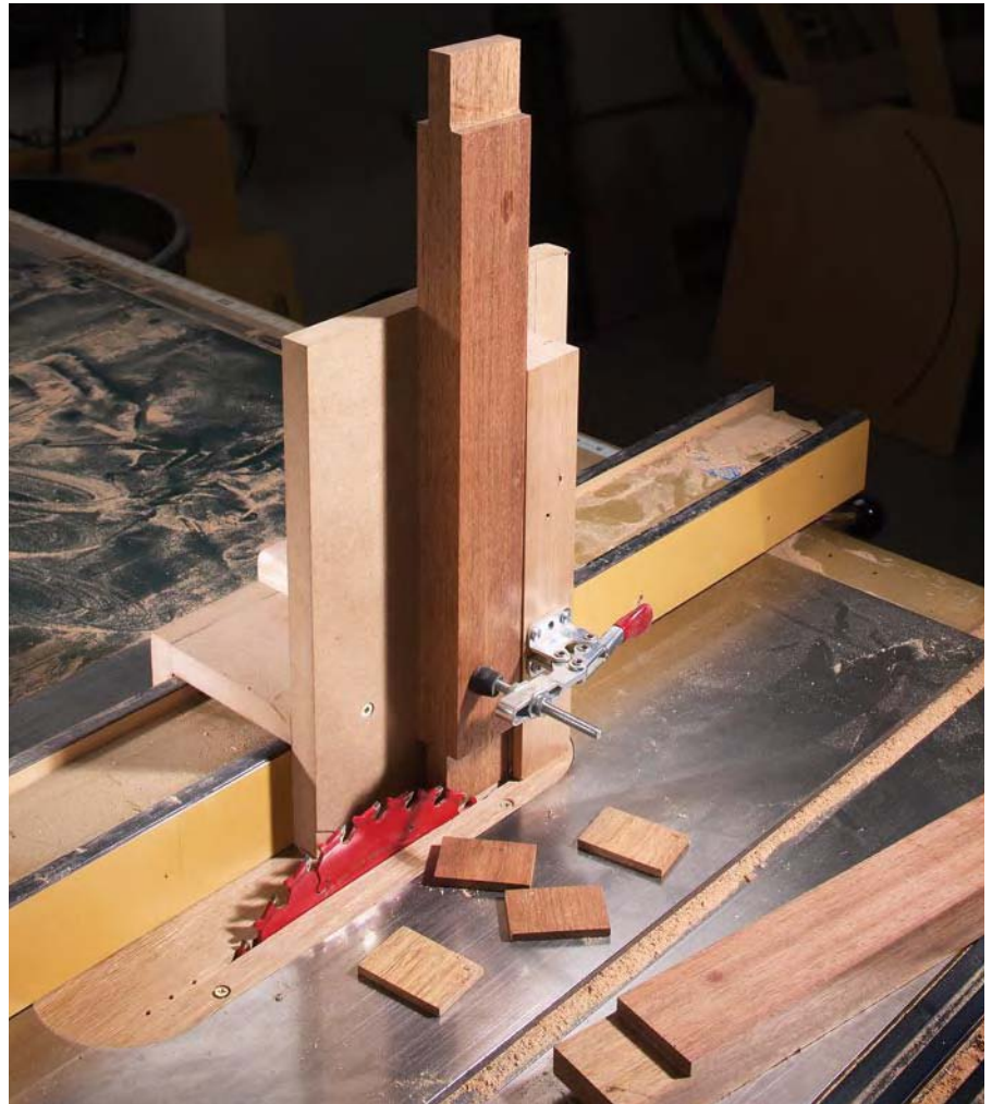
Nothing wrong with simple. This tenoning jig performs one task, and does it safely and accurately. It costs little, and makes use of the existing table saw fence for fine adjustments.
