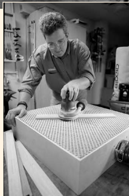
A down-draft table is a great way of capturing airborne dust. Connected to a portable collector, this table will pick up dust the sander's integral dust collector is bound to miss.
