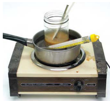
Heating options. You don't need to invest in a glue pot. Any situation you can arrange that will keep the glue at about 140° to 150° will work well – in this case a jar of glue in a pan of water on an electric hot plate. Keep an eye on the temperature.
