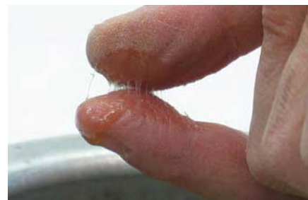
Finger test. Rub joints work well with hot hide glue because of the strong tack created when the glue cools to about 95°F. Use your fingers to check the strength of the glue as it ages and loses tack. The glue cleans off quickly in hot water.
