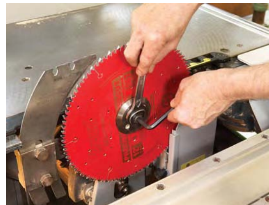
Pop the hood. You change the blade by sliding the table back, giving you lots of room to work. At the bottom right of the blade is an adjustable shroud that attaches to the dust-collection system.
