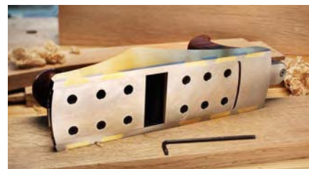
Sole of a new machine. The VP-60 has two sole plates to close up the mouth for any planing situation.
