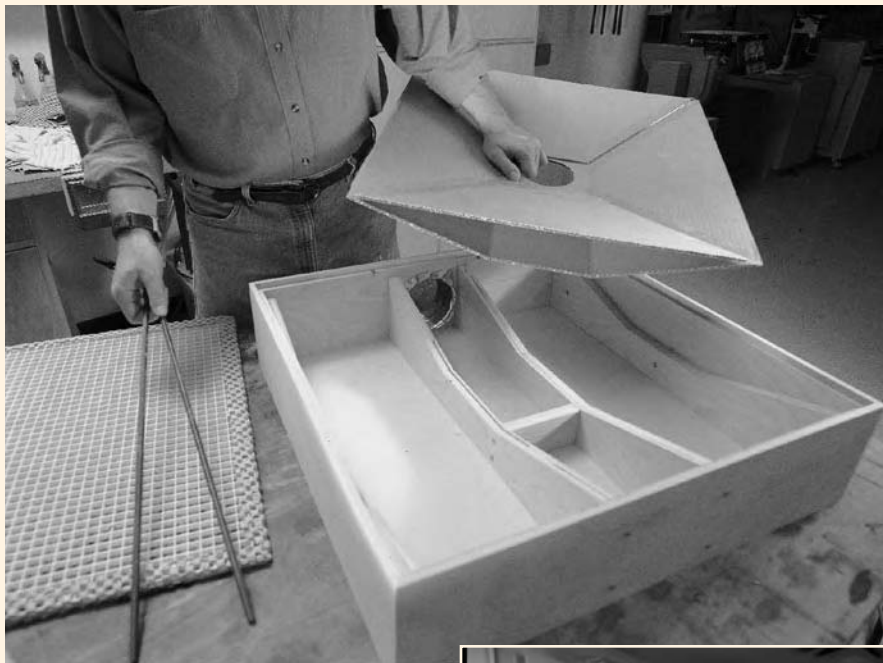
A down-draft table is a great way of capturing airborne dust. Connected to a portable collector, this table will pick up dust the sander's integral dust collector is bound to miss.
