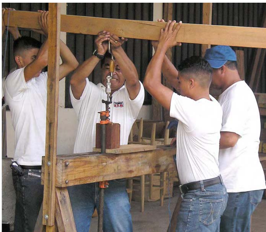
Old-fashioned ingenuity. The beam drill in action. The downward force provided by the beam above the brace assists greatly in boring accurate holes.
