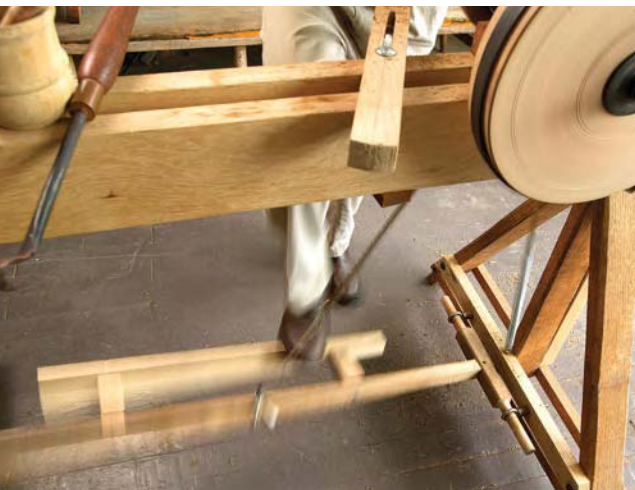
Fancy footwork. I press the foot pedal down to the floor and that pulls the chain down with it ...
