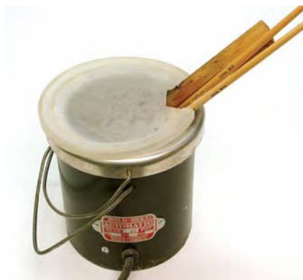
Keep it covered. A commercial glue pot maintains the temperature of the glue at an ideal 150°. To retard evaporation and the glue thickening, I keep the pot covered with a plastic lid. The lid has a cut out for brushes and a stirring stick.
