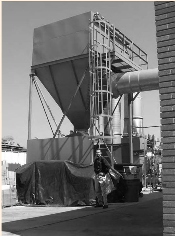
This gigantic dust collector services a big woodworking shop at Cerritos College in California. Small shops can use the same type of equipment – only a lot smaller in size.
