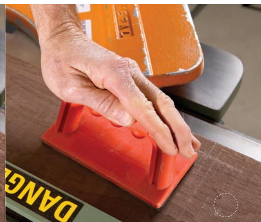
Wrong and right. The push blocks that came with your jointer are useful if you use them correctly. Don't grasp the handle as shown above left. This traps your hands. Instead, wrap your hand over the push block as shown at right. Don't forget to replace the pad's foam with a piece of sandpaper.
