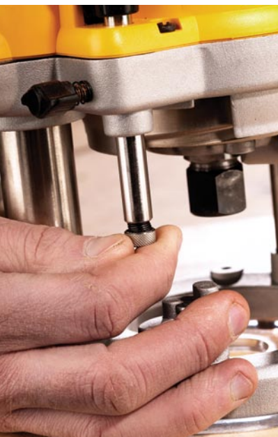
A fine-threaded nut at the end of the plunge rod makes fine-tuning depth settings simple and precise.
