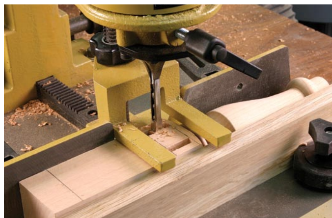
The lower front rail connection is a twin mortise and tenon. The mortiser setup is identical to that for the sides. Simply reverse the leg to cut the second slot of the mortise.
