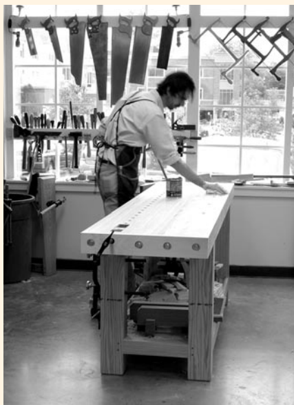
An oil-varnish blend (any brand) is an ideal finish for a workbench. It resists stains, doesn't build up a film and is easy to apply. Two coats are all I ever use.
