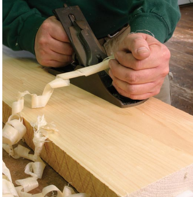
The result of your labor: The shaving emerges from the center of the mouth and clears the tool easily without clogging.
