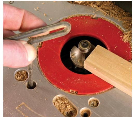
Above-the-table adjustments aren't always as easy as they seem – the hole to reach the screw can fill with debris, and you'll likely need to bend down anyway to see the edge of the bit.
