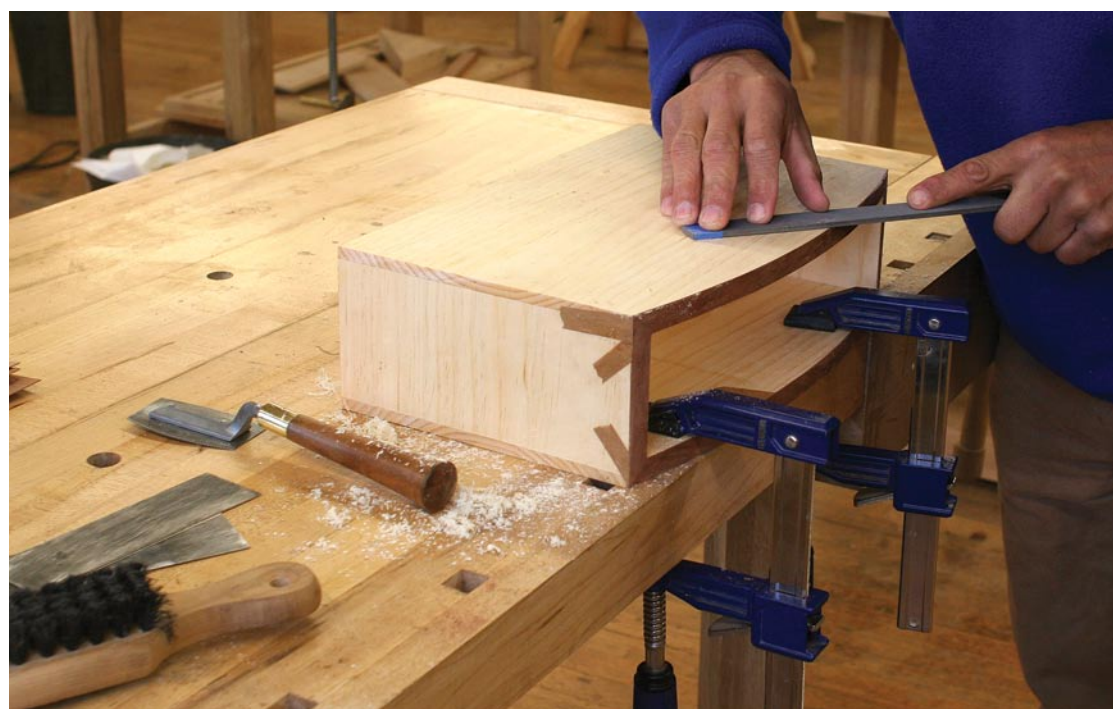
Holding a mill file flat to the surface produces a clean edge without any "rolled" edges.
