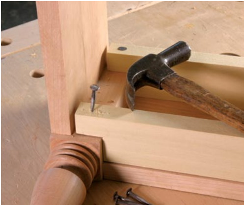
The runners and kickers can be set square off the front of the base and nailed to the rear leg posts. Drill a pilot hole through the pieces but not into the leg. Drive the nail at the pilot hole to gain a strong hold into the leg.
