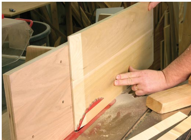
Set the saw blade to 12° and leave a 3/16" space between the blade and the fence. The resulting cut will fit perfectly in the 1/4" x 1/4" groove for the drawer bottom. Raise the blade to make a clean cut.
