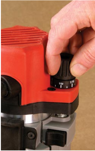
The Milwaukee's fine adjustment on its fixed base was the favorite of the routers tested.
