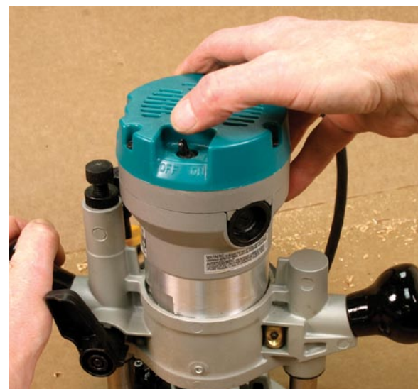
For some switches, such as on this Makita, it's necessary to remove one hand from the router to reach the switch.
