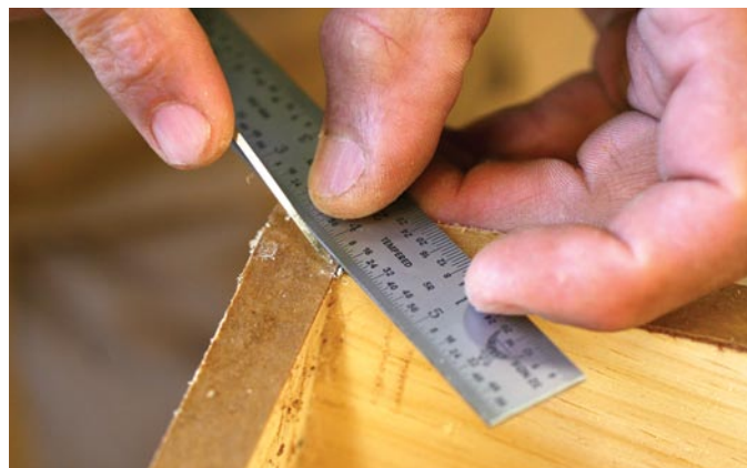
Lay a ruler across the points of the miter, then cut through both layers with several passes of a sharp marking knife.
