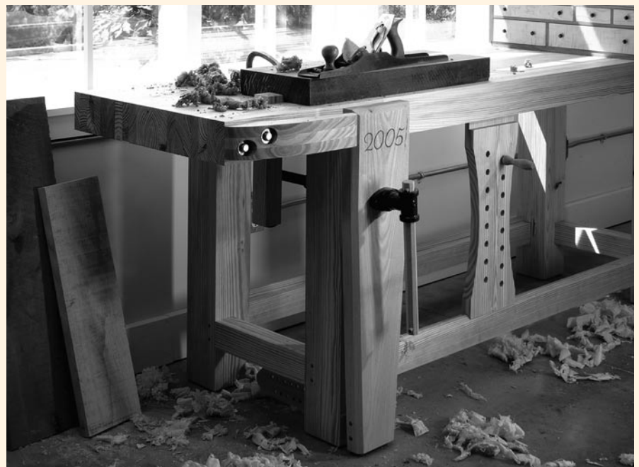
This French-style workbench weighs more than 325 pounds. The top is 4" thick. The legs are 5" square. All this mass absorbs vibration and makes every cutting operation smoother.
