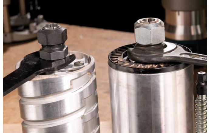
The large cast wrench of the Milwaukee (right) made for easy bit tightening. The thin stamped wrench of the Makita (left) tended to slip off the nut.
