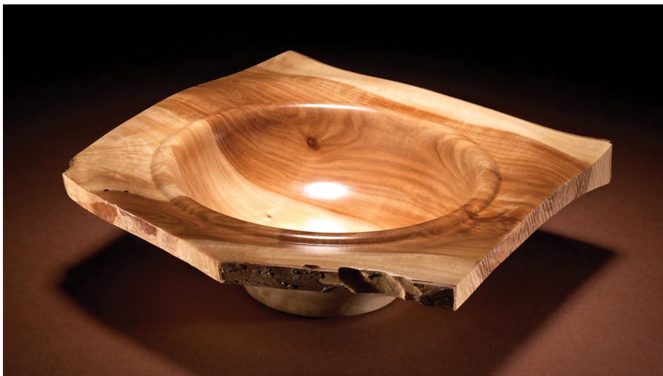
A “square” bowl is turned using the saw cuts and the outside edges of a chunk of wood as the edges of the bowl itself.
