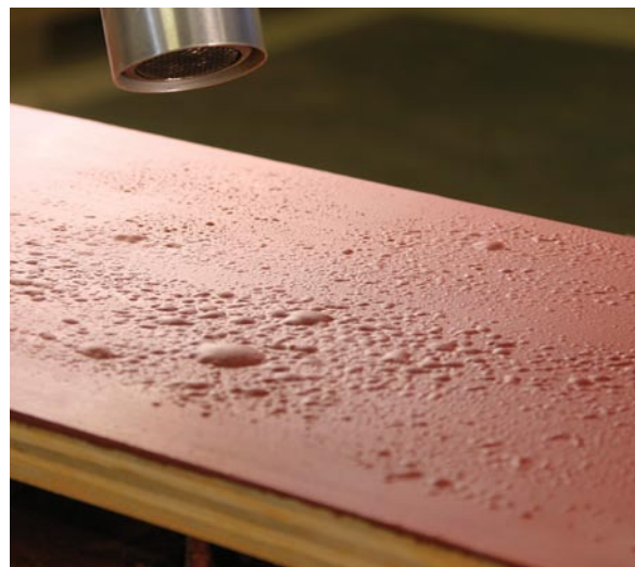
After another coat of lacquer and then paint, blister the top color with your heat gun. The more blistering, the more base color will show through.
