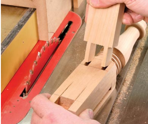
Once the insides of the twin tenon are nibbled away you can test fit the joint. Make it snug but not tight.
