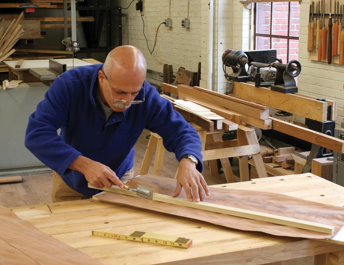
Several strokes with the veneer saw held against a straightedge will create a clean edge on the veneer leaf.
