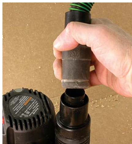
The Porter-Cable, as well as the DeWalt have the dust collection attachment at the top of the column, a more convenient location.
