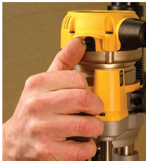
The switch on the DeWalt is in an easy-to-locate, and easy-to-operate position.
