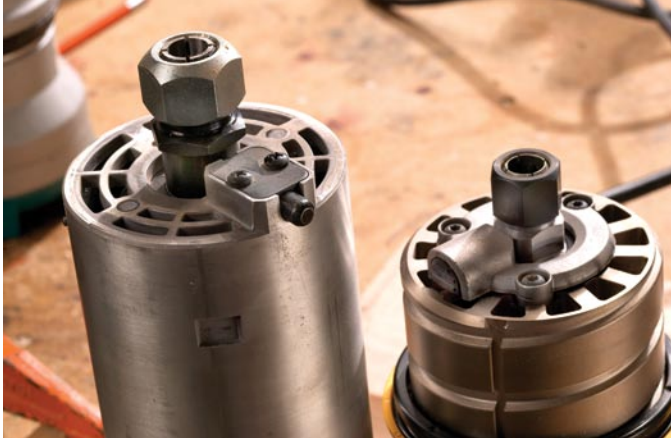
Spindle locks sound convenient, but they all had problems. The Ridgid (left) was easy to operate, but in the way when changing bases. The DeWalt was difficult to press in.
