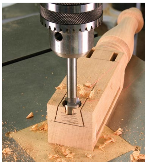
Define the dovetail socket with your handsaw, then "hog out" much of the waste material with a Forstner bit at the drill press. Finish with your chisels.
