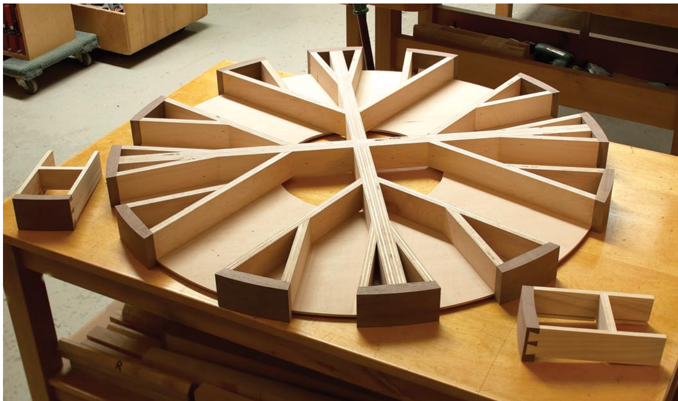
Stacking the deck. Plywood strips on a maple-veneered MDF base form the intricate structure of the tabletop.
