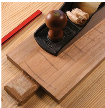
First marks removed. After taking the first two passes with the plane, the pencil marks at the edges of the board are removed. Now place the center of the plane on the line where the pencil disappears and take another pass.
