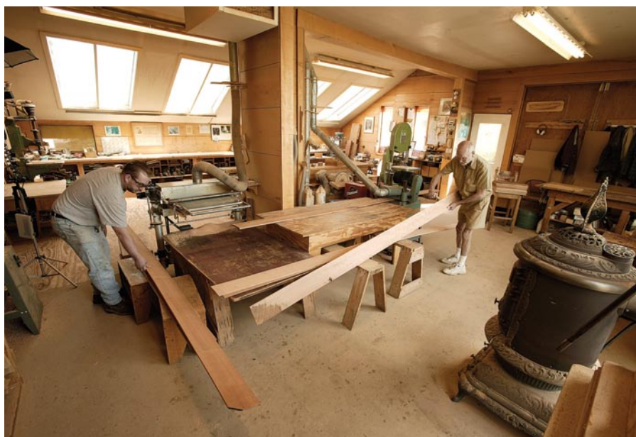
Re-purposed. Recycled sliding-glass doors serve as skylights, flooding the shop with natural light.
