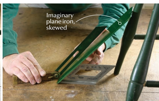
On the diagonal. As you can see in these pictures, moving slightly at a diagonal across a surface actually presents a lower angle of attack, and helps to prevent tear-out.
