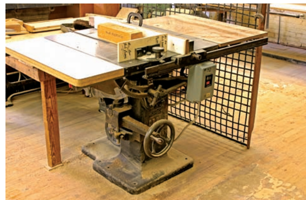
This is your grandfather's table saw. Box lids are separated from cases on this vintage saw. Sound construction and constant maintenance keep many old machines in use.
