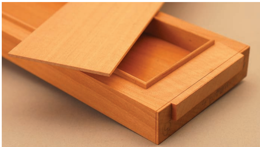
See the sawn details. Above is shown a sample of thin solid veneer. In this case it has been used for a small box lining in one of my student's work.
