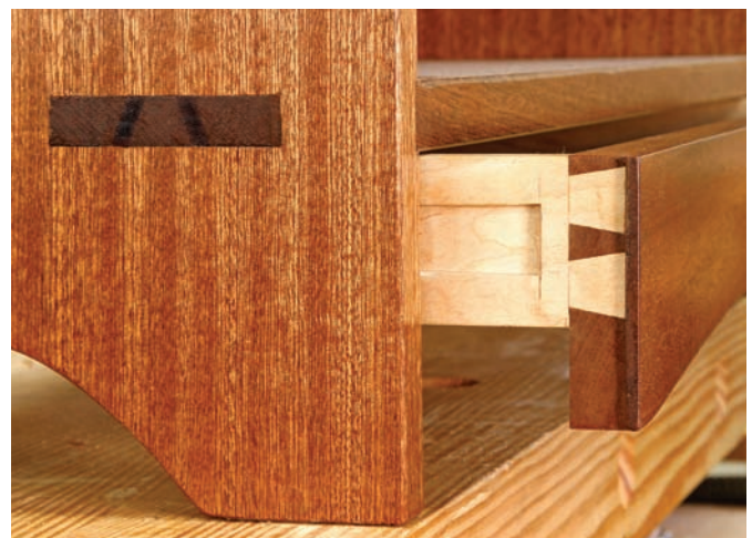
Now you see it. The rabbet in the end of the drawer front provides clearance for the sides, while allowing a narrow margin to be trimmed easily.
