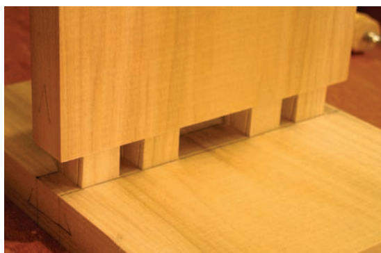
Test run. Do a dry fit (without wedges) to ensure the pieces fit snug, and clean up your cuts as necessary.
