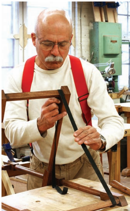
Clamp in position. Leg assemblies are clamped to the bench before webbing is tacked to the upper rails to hold the legs in the open position.
