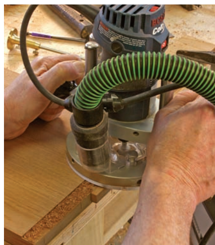
Shoulders first. A shallow rabbet is cut on each side of the shelves to start the making of the tenons.
