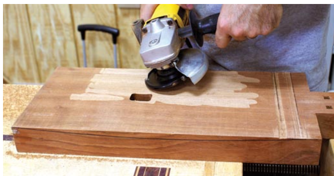
Let the chips fly. An angle grinder and a carving blade make one powerful combination! Hold the tool close to horizontal to avoid sculpting deep gouges.
