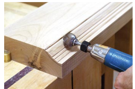
Big coves, no problem. A hand-held die grinder with a ball mill is the tool of choice for creating large coves.
