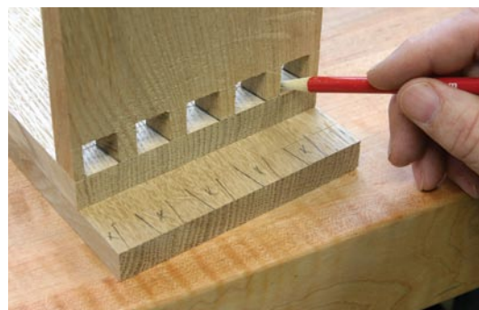
Sharp lines, tight fit. Align the top onto the clock sides, use a sharp pencil to transfer the lines and mark the waste area to be removed. The extra marks assure that you'll waste the correct area.
