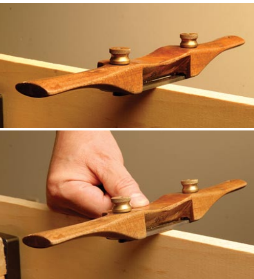
Training. Set the shave flat on your work, then place your thumb in the curve to slightly increase the angle; that's the correct angle for use.
