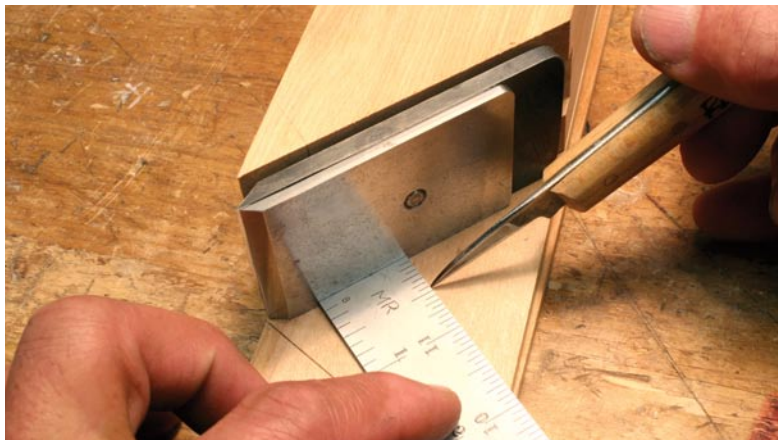
Critical location. Carefully measure and mark for the cross bar.
