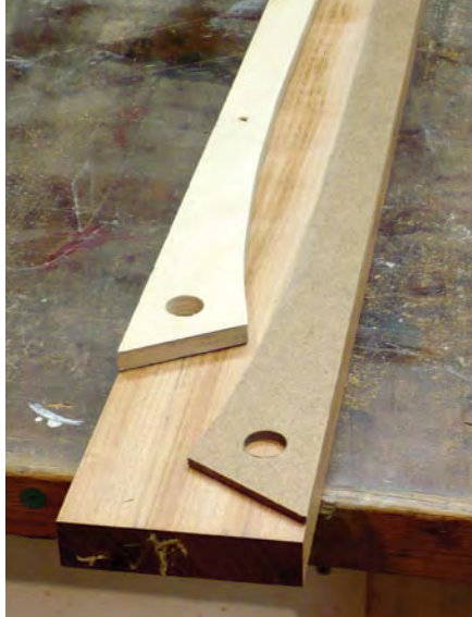
Start with a blank. A 6"-wide blank is ideal for laying out the slats so you can nest the parts.
