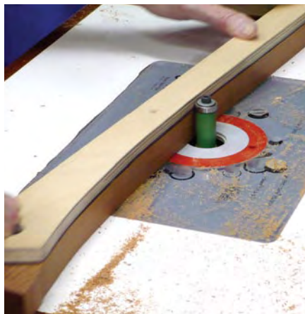
Pattern-route the slats. Jatoba is very brittle and prone to splintering, so attention to grain direction while routing is essential to avoid tear-out.
