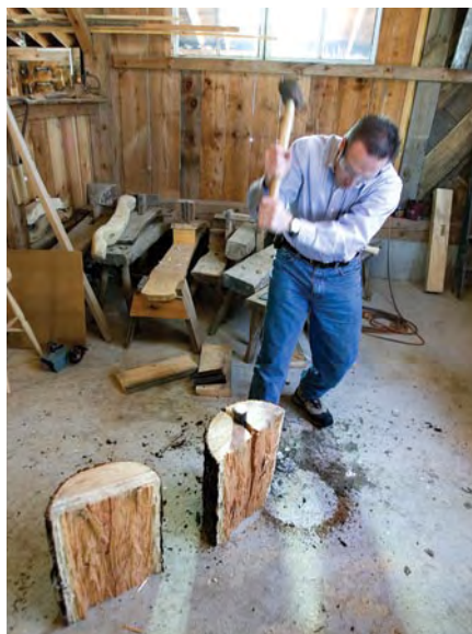
Power tool. Author Jeff Skiver tries his hand at one of mankind’s original simple machines as he uses a wedge to split log sections into more user-friendly chunks of wood.
