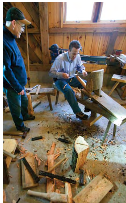
A close shave. A shaving horse holds a hewn leg blank in place as Skiver roughs out the shape prior to turning. Instructor Dave Abeel looks on.
