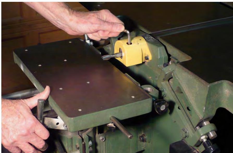
Horizontal mortises. I used the horizontal mortiser with a ½" spiral upcut bit on my Robland X-31 to machine the mortises in the legs
