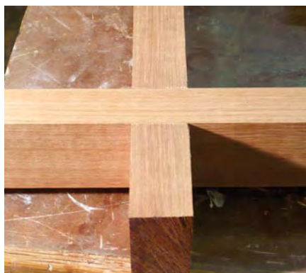
Tight is key. Strive for a snug fit between the stretcher and lower rail.
