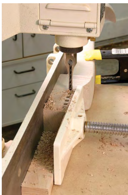
Leg support. To cut the mortises into the legs, you need to add support under the top block so the knee is off the table. Add a small wedge below the knee to stabilize the piece.
