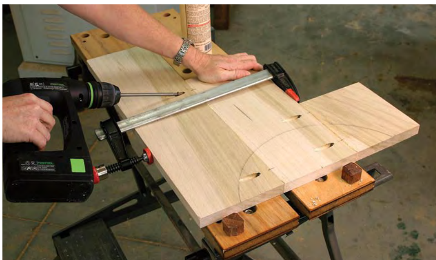
How to be clever. The online manual helps you figure out how to do many complex operations with simple tools. You don't need 10 clamps to create a flat panel. One clamp and a few well-placed screws do the job nicely.
