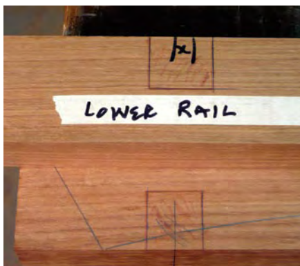
Mark the notches. Carefully mark the notches for the rails. Here, a lower rail blank is lying on top of the stretcher blank.
