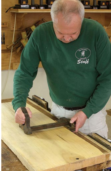
Panel gauge. A panel gauge is simply a large marking gauge that is used to scribe a line parallel to a jointed edge.
