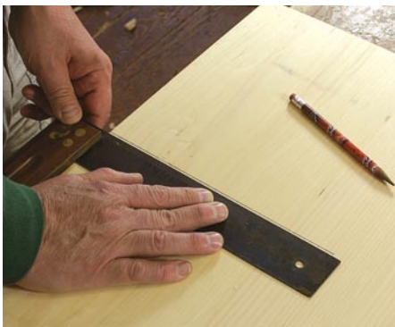
Try square. An easy test to see if your square is indeed square is to place it on a proven straight edge and draw a line. Now flip the square so the handle is pointing in the opposite direction, and see if the tool confirms the line. If it doesn't, buy a new square.
