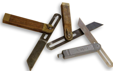
Bevel squares. There are several types of bevel squares, all of which are handy for laying out angles, but also for measuring unknown angles.
