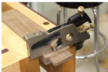
A shoulder to lean on. The shoulder plane allows you to fine-tune the fit of your tenons, one wispy shaving at a time.
