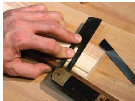
Bottoms up. I know I'll have to plane the tops of the aprons, so I used the bottom as the reference face. Unfortunately, the moulding prevented me from accessing this face directly. But sticking moulding after you've cut the angled tenons on the end can be a drag. So I'm using my straight-edge to help.
