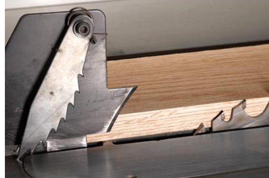
Tooth trajectory. In the top photo you can easily see the trajectory of the blade’s teeth and the closeness of the blade to the splitter. Above, the teeth trajectory is forward, toward the operator and the distance between the blade and the splitter has widened.
