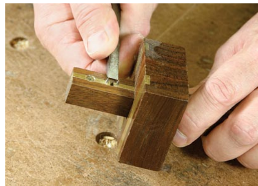
Mortise gauge. If you hand cut mortises, a good trick is to set your mortise gauge to the width of your mortise chisel.
