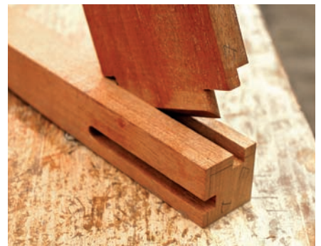
Long as I can. To maximize the length of the tenons in the rear legs, the ends are mitered.
