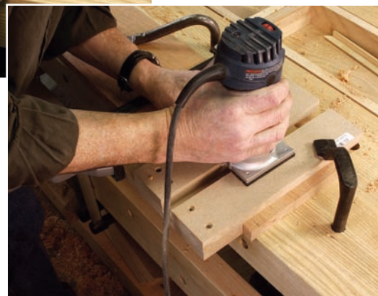
Stop action. A pencil mark indicates the end of the dado, and because the router will leave rounded ends, I stop just short of the mark.
