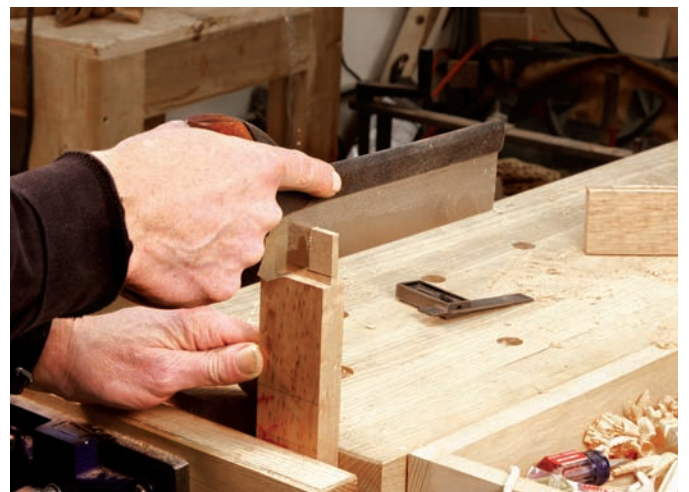
Faster by hand. Cutting the haunch by hand is faster than setting up to make these cuts by machine. Only the end of the haunch will be seen in the finished door, so this is a good place to practice making cuts by hand.
