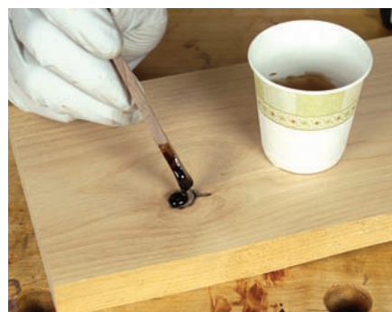
No longer loose. Stabilize knots and make them look natural with epoxy and dye.
