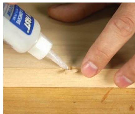
A quick fix. Accidental chip-out can be reattached in seconds with quick-drying CA glue.
