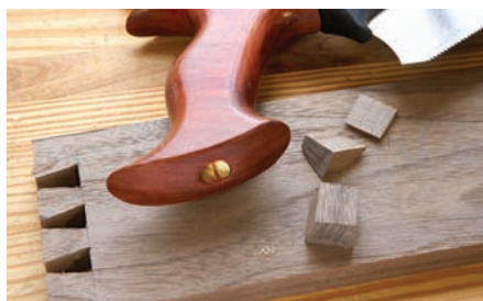
Simple connection. A single bolt connects the handle to the spine and blade—a cost-effective solution to a labor-intensive process.
