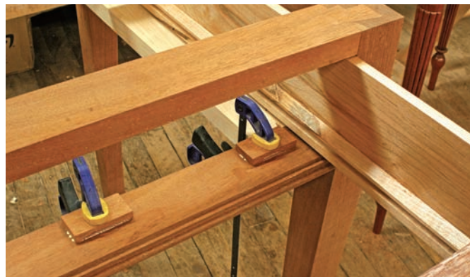
Stop right there. Assembling and fitting the drawer before installing the drawer bottom allows precise placement of stops glued to the lower rail.
