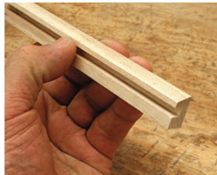
Smooth transition. The angled top of the slip bridges the corner between the sides of the drawer and the bottom.
