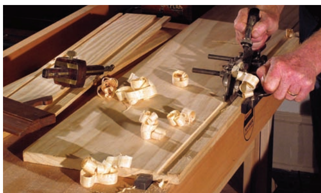
Mark and make your groove. The first joinery is making the interlocking grooves in the pieces for the skirt and top section of the chest. Mark their locations with a mortising gauge first to increase your accuracy.
