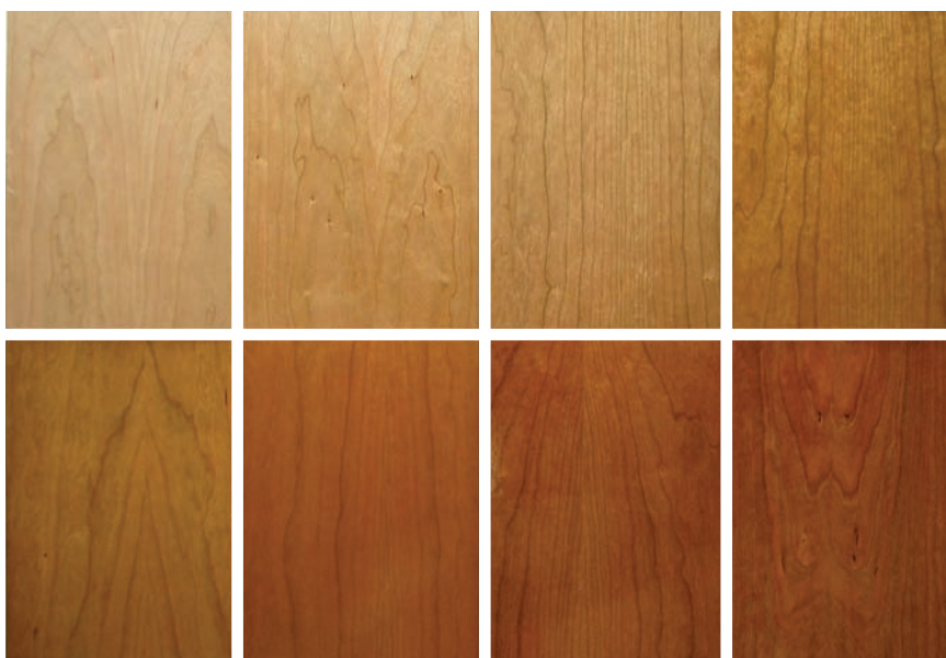
Seven finishes on cherry. Top row from left: unfinished, clear paste wax, water-based finish, nitrocellulose lacquer. Bottom row from left: clear/blonde shellac, amber/orange shellac, polyurethane varnish, boiled linseed oil.
