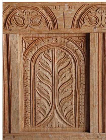
A shaped carving. In this reproduction of a William Savell chest, the carving is executed first with V-tools to define the shapes, then gouges to provide a more shaped appearance to the carving.
