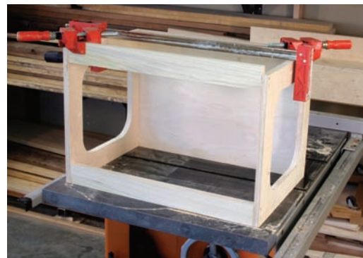
Start flat to end flat. Assembling the frame on a flat surface makes it easier to align parts, and ensures a flat surface for mounting the top.
