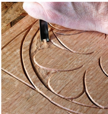
The completed outline. Here's the finished outline of the panel, which was completed entirely with a V-tool and a few simple layout lines.
