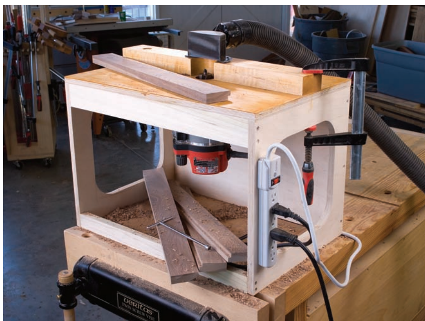
Not fancy, but functional. A good router table features a flat, solid top and a straight fence. With those in place, there isn't a need for much more.
