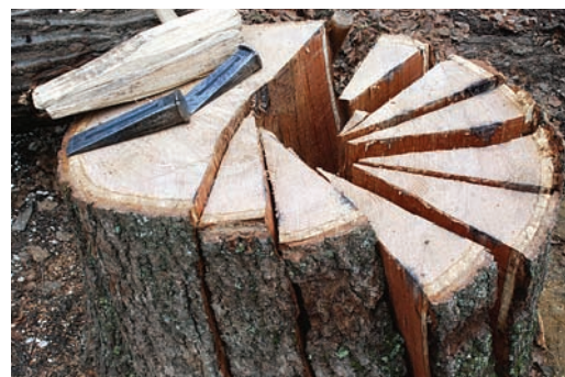
Splitting the stock. I've split half an oak log into 16ths, to be split again into 32nds. Each wedge shape is truly radial. It's very stable and, when squared, extremely satisfying to work.
