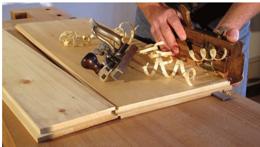
Make a stout bottom. A tongue-and-groove joint in your bottom boards ensures the longevity of your chest.
