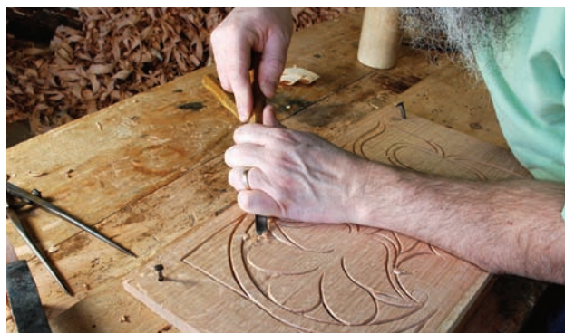
Remove the background. Remove the background using a shallow gouge driven by hand pressure. Here, my left hand is bracing the tool and my right is pushing it into the cut.
