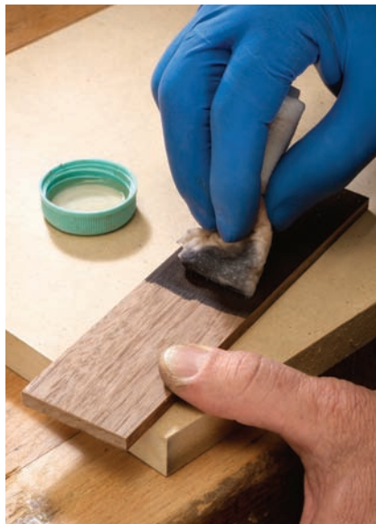
Iron-on color. Above, I'm wiping the first iron layer onto tea-saturated walnut.
