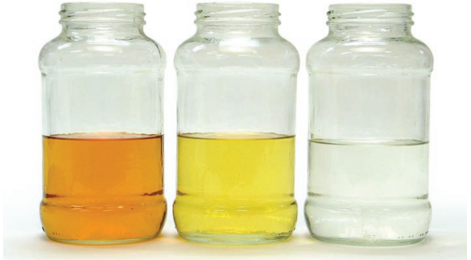
Color. When poured into glass jars, it’s easy to see the different colors of lacquers. On the left is nitrocellulose, which is made with fairly orange modifying resins. In the middle is water-white lacquer, which is made with fairly colorless modifying resins. The color that exists is supplied mostly by the nitrocellulose. On the right is CAB-acrylic lacquer, which is totally colorless.
