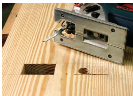
No mortiser required. With large through-tenons you can simply drill a starter hole for your jigsaw's blade then square things up. Don't rush the cut or the blade will deflect.
