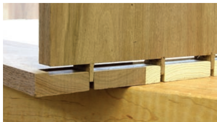
Disappearing joinery. Form the tails in the case bottom after you cut a rabbet \frac{1}{8} " below the inside surface. This allows the base moulding to cover the dovetail joint.
