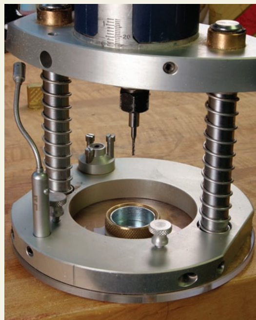
Stretching the point. Collet reducers, chucked into regular collets, can help to lengthen a router bit's reach.
