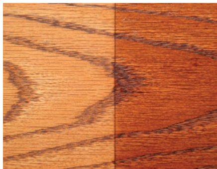
Oil stain vs. dye. Oil stain (left) doesn't color the dense parts of oak as well as dye stain (right).
