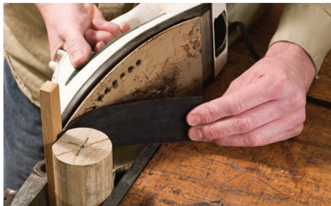
Tailor-made veneer. Using moisture and heat to bend the outer layer of black veneer is as easy as pressing a collar.
