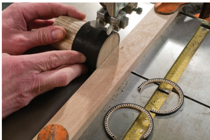
A wee-bit thicker. Individual rings are sawn oversized at the band saw, then planed, scraped and sanded flush.
