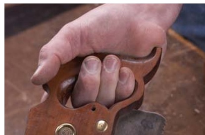
Discomfort grip. If the horn digs into your palm, you won't be able to saw comfortably – and you'll try to overcome the pain by changing your grip (to the wrong grip).
