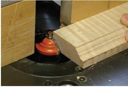
More for the money. Additional cutting surface beneath a bearing is valuable real estate and required to gain the needed profile.
