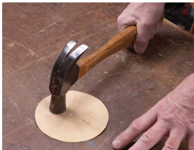
Sandpaper test. Swing your hammer to hit a piece of sandpaper – the strike should happen when the handle is parallel to the floor – to see where on the head you're hitting. If it's not at the apex of the bell, you're in danger of dinging your work, and you should adjust the head as needed with coarse sandpaper.
