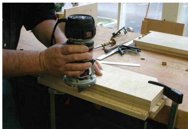
Power & hand. Assemble the box, mark the start and stop points for the door rabbet, then clean the bulk of the waste using a router. Chisels fine-tune the work.
