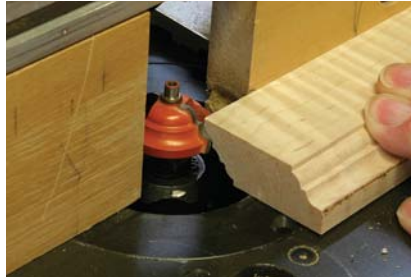
Second position. After a height change and fence adjustment, the profile is complete using a portion of the bit.
