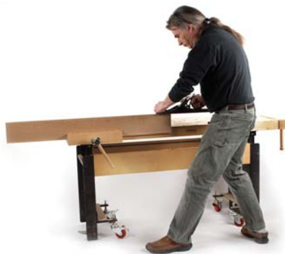
Freedom to control. When the arms and hands don't do the heavy work, those muscles are available to control the position and pressure of the tool.
