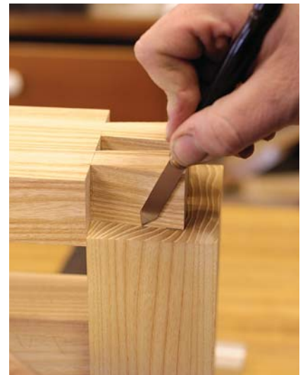
Shift right, scribe left. Scribe lightly. You don't want to make a grand canyon here.
