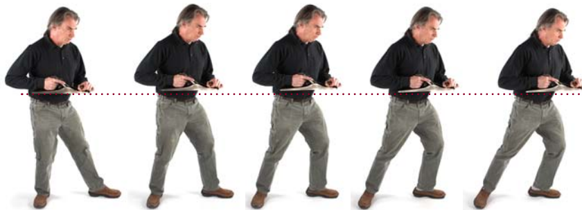
Fundamental move. Shifting my weight from one leg to the other allows me to keep my arms and hands in position. At the start, all my weight is on my back foot, with that knee bent for balance. As my weight shifts, I straighten that knee and bend the other one, ending with all my weight on the other leg. My hands and arms move in a nice straight line.
