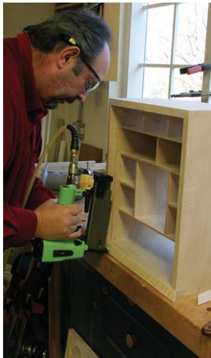
On the level. To keep mouldings aligned, work with the box and mouldings placed directly on the bench. Remember: Mouldings attach to the box, not to the bench.
