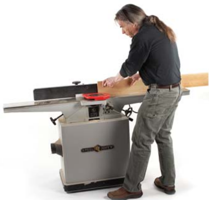
Power tools, too. Shifting weight to provide motion provides consistent control at the jointer, as the feet take a step and walk through milling an edge.
