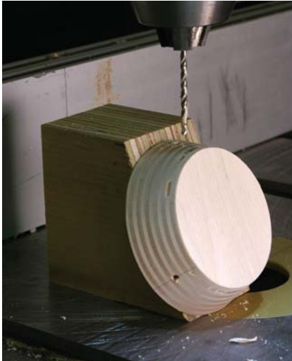
Holes for hardware. The edge is angled at 22.5°. Cut that angle on a piece of scrap and hold your small disc against it. Line up your layout line with a line on your scrap or (in this case) a lamination line in the plywood.
