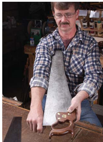
A little short. This 26" saw is a little bit too short for me – but 26" saws are much easier to come by in the wild than 28" saws, so sometimes I'm forced to make do – and I can tell you, it's not as efficient.
