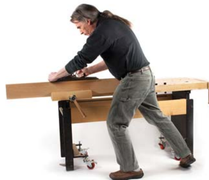
Freedom to control. When the arms and hands don't do the heavy work, those muscles are available to control the position and pressure of the tool.
