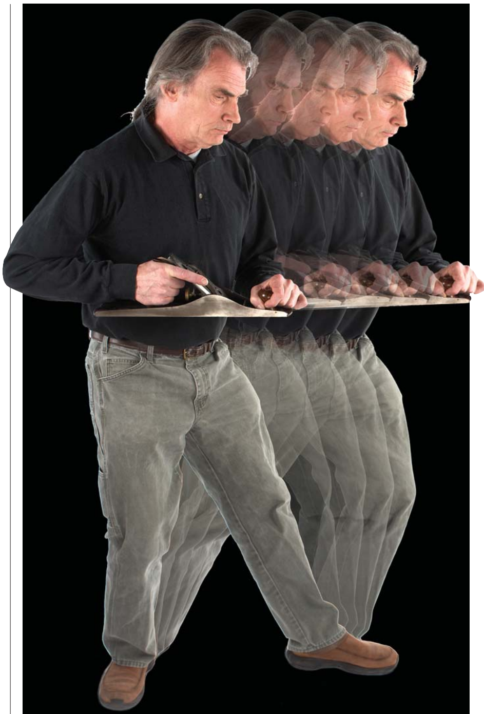
Hands steer, legs move. Proper movement is key to using your body effectively when you work.
