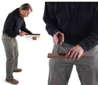
See the curve. Sawing directly from the torso puts the parts of the arm at odds with each other. When they move, it won't be in a straight line.
