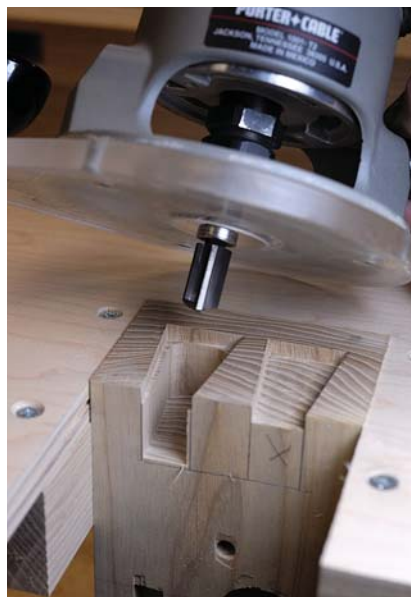
First pass. Get rid of most of the waste on your first pass.
