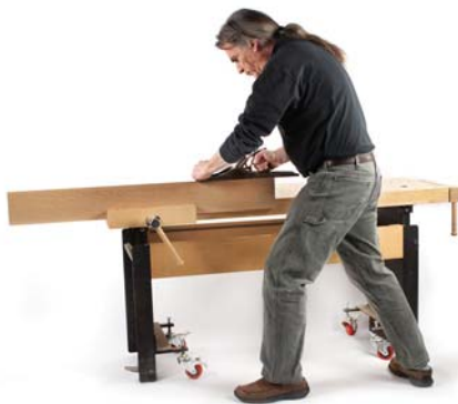
Freedom to control. When the arms and hands don't do the heavy work, those muscles are available to control the position and pressure of the tool.
