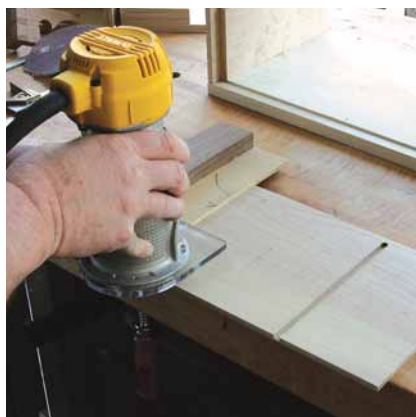
New mark. Divider dados stop \frac{1}{4} " short of the shelves. Use the same jig, but adjust the stop-cut mark.
