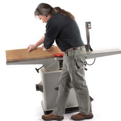
Power tools, too. Shifting weight to provide motion provides consistent control at the jointer, as the feet take a step and walk through milling an edge.
