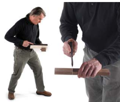
Feel the line. Turn and change your stance, and the parts of the arm naturally line up. From this position the arm swings in a nice line while staying relaxed.
