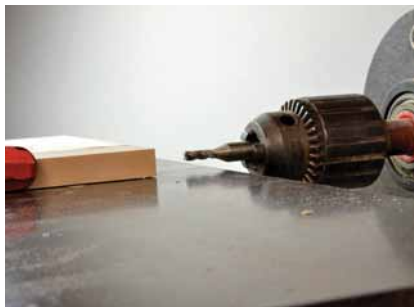
Floating tenons. A horizontal boring machine cuts the mortises for my floating tenons.
