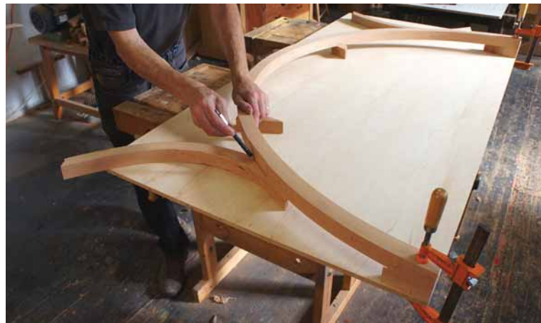
Full-size layout. A piece of plywood locates the corners of the large arch and the wings. Mark the wings from the flats on the arches.
