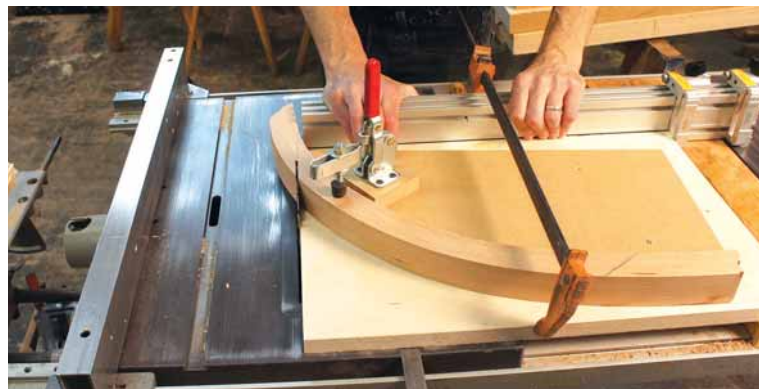
Safe & secure. The jig holds the curved part securely to make the cut, creating a flat surface to attach the wing to the arch.
