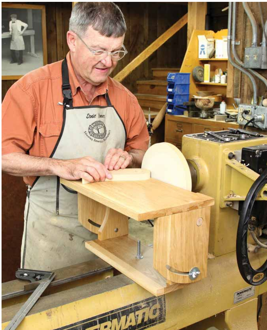
Your $50 disc sander. Just about any lathe will provide the power and the platform for a shop-built disc sander. It also has some extra features including variable speed and little, if any, vibration.
