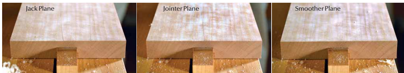
Leaving tracks. Here you can see the progression of track marks from blades ground and sharpened straight across. With overlapped plane passes set to take a .0015"-thick (or thinner) shaving (right), the tracks disappear.
