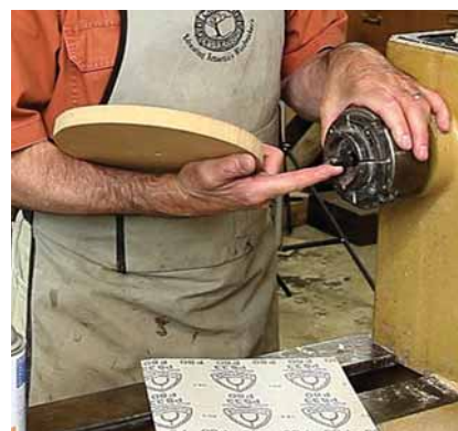
Affix your sanding disc. You can mount your platen or sanding disc to your lathe spindle using a face plate or a four-jaw chuck with a screw, as I'm doing here.
