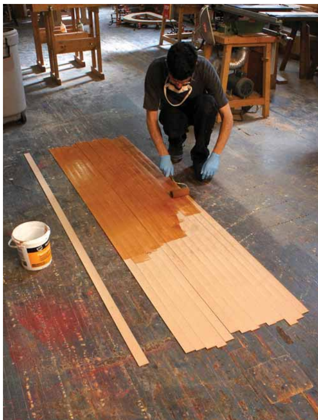
On a roll. A paint roller makes quick work of spreading the glue evenly on all of the laminations.
