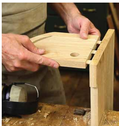
Glue up your parts. Use whatever method you prefer to join the base to the stanchions and the table to the sectors. I used a Festool Domino machine.
