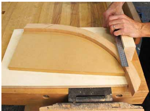
Let it ride. Align the straight cut on the wing with the edge of the jig base.
