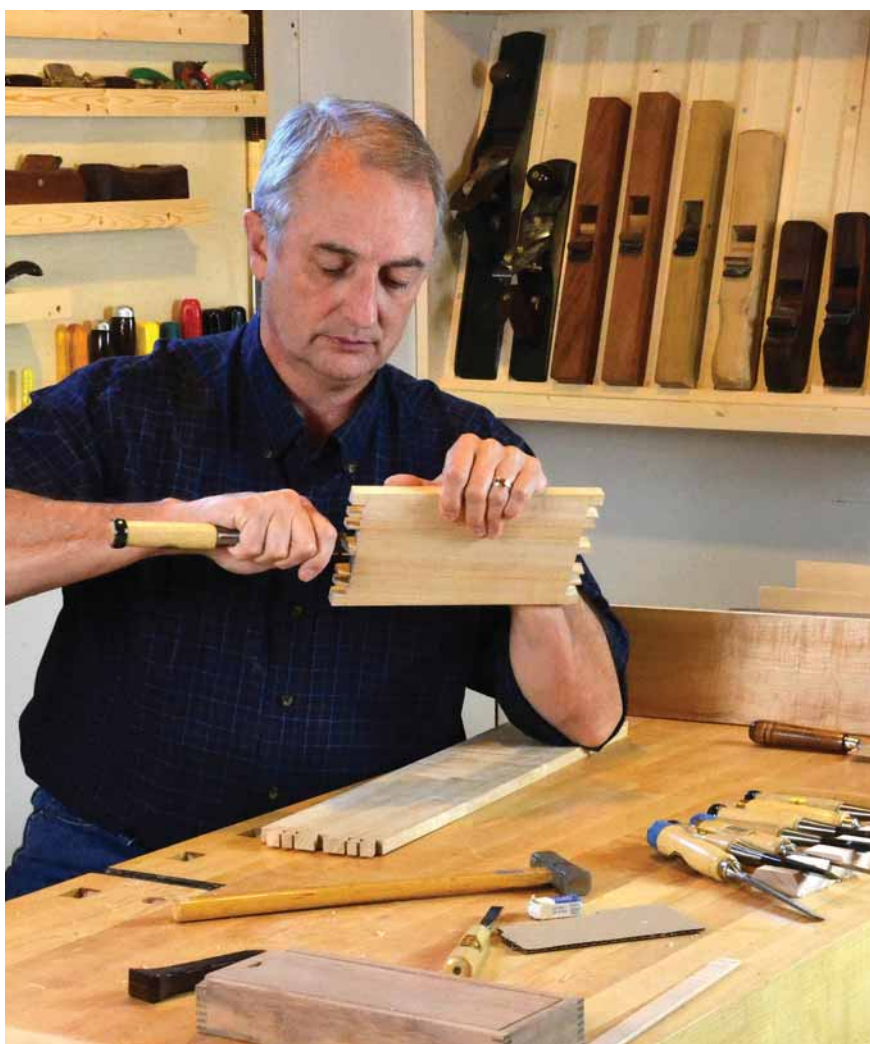
Pare. Tune your pins with a sharp chisel for the perfect shape before transferring the shape to your tail board.
