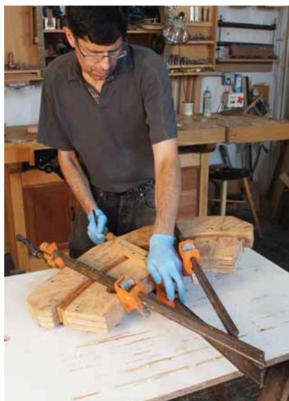
Caul of the wild. A form for the outside of the curve helps to spread clamp pressure, reducing the number of clamps needed.
