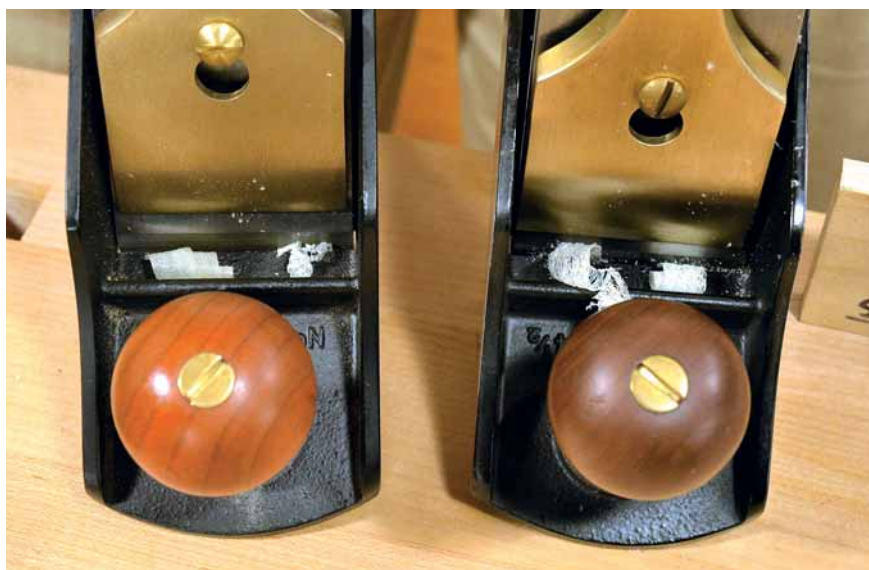
Test. In the plane on the left, you can readily see that the two test shavings are different thicknesses; this tells you the blade is not parallel in the plane's mouth. On the right, the two shavings are the same thickness, which indicates the blade is properly aligned.
