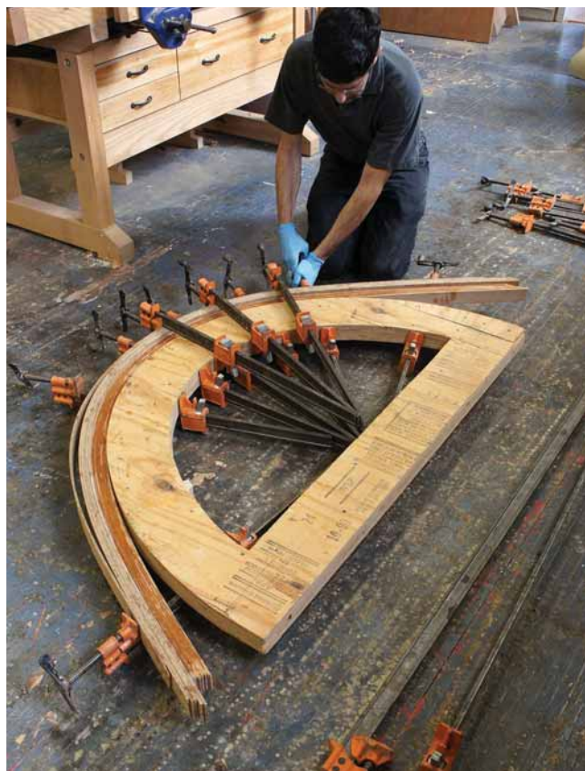
Practice first. Before you add glue, do a dry run to ensure you've enough clamps – and that when the glue is on, you know where to place them.
