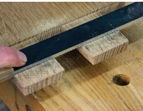
Off the top. The pencil marks indicate the high spots. Remove them with a float, then test the fit again.
