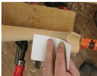
Upper marks. Using poster board as a flexible straightedge, mark the upper portions of the center toe.
