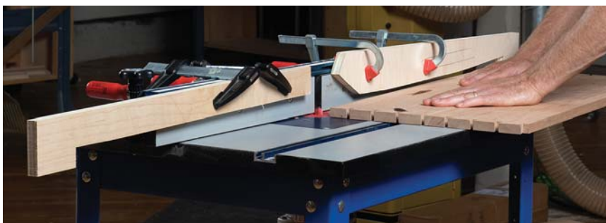
Stop that rabbit. Set up stop-blocks on your router table's fence to register the front and back as you mill the rabbets in the back inside edges of the case sides.
