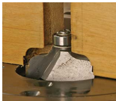
Locked-in design. Router bit profiles limit design possibilities and often are not appropriate to a period design.
