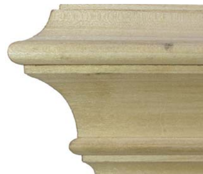
Sensible sequence. Hollows and rounds allow you to produce well-proportioned complex mouldings with a few simple tools.
