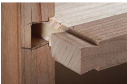
Dovetail socket. The socket for the case dovetail is located at the end of a shallow dado that houses the drawer divider.
