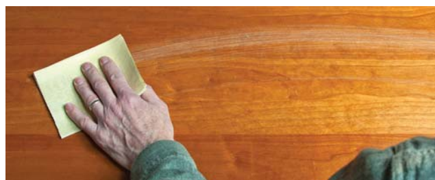
Natural arc. The natural pivoting motion of the shoulder leads to a curved sandpaper path if you sand from side to side. For straight strokes, reposition the work (or yourself) to sand out from and back toward your body.
