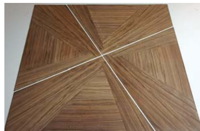
4. Quadrants. Work on the overall pattern in quadrants, repeating the shoot then glue-up process until you have four workpieces.
