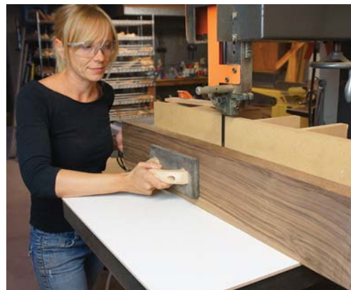
Saw your own. Resawing your own veneer allows you to control the thickness and grain pattern to suit specific goals.
