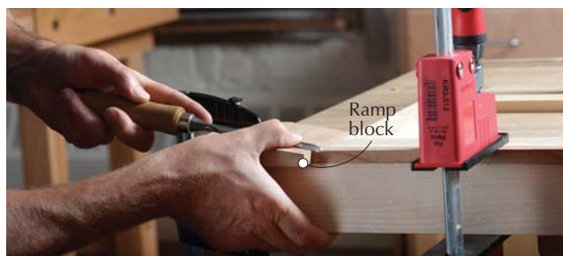
Guided chisel. As an aid to cutting the dovetails on the divider fronts, use a shop-made "ramp block" to guide the chisel and help achieve consistent sizes and angles.
