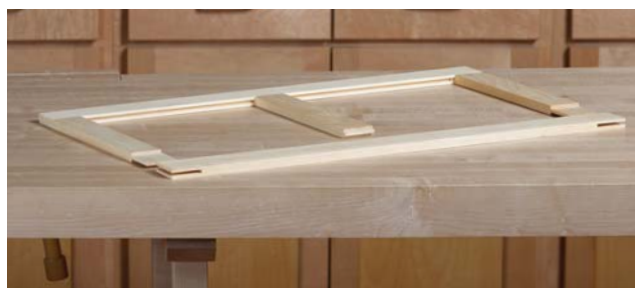
Frame-up. The case is divided using frames with slip joints at the ends and stub tenons where needed for a center divider. These frames support the drawers and fit in dados.
