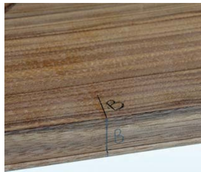
Registration. Mark where your veneer glue-up meets the substrate, and make sure you can easily see the marks.
