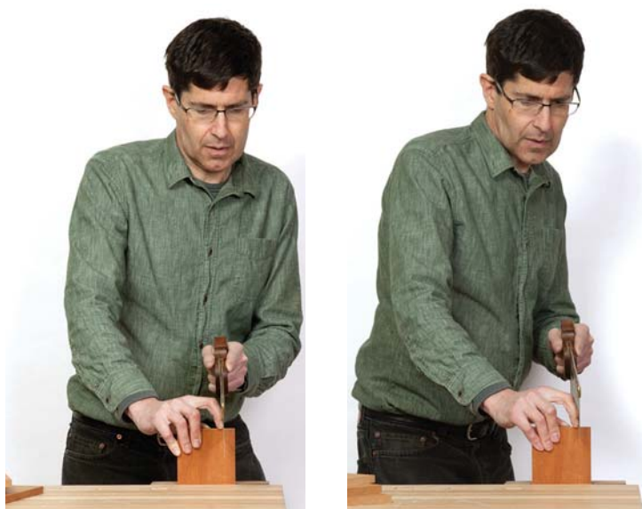
Alignment counts. Put your body in front of the saw (left) and you force your wrist and shoulder to move out of alignment with the tool in order to make a straight cut. Instead, align with the saw the parts of your body that are in motion.
