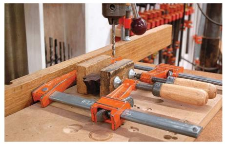
**Drill after shaping.** If you neglected to drill holes for your screws or pins before shaping your handle, clamp it tightly between blocks to hold it square.
