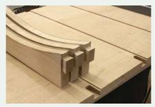
Don't fret it. As with the earlier dovetails, the drawer-blade joinery is concealed in later steps, so you could add wedges to tighten any problem spots.
