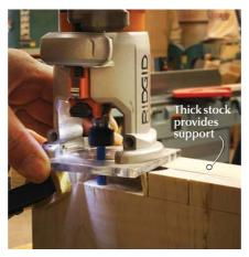
Waste removal. Socket waste is quickly removed with a router. I get added support using thick stock clamped to the work. Rout close to your lines then use a flush-cut saw to remove the last slivers of waste.
