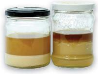
**Thinned varnish separates.** Oils, varnishes and oil-based polyurethanes separate when they have been thinned with green paint thinner. You have to shake or stir before using any of these finishes if you have thinned them with green paint thinner.
