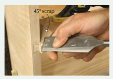
Miter your bead. The best way to miter the small ends of the drawer-blade bead is to use a mitered scrap to guide a chisel as you pare.
