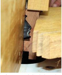
**Under pressure.** Featherboards, above and in line with the cutter, provide the necessary pressure where it is needed most. They also encase the rather large moulding bit spinning inches above the table. A push stick is used at the end of the cut.
