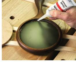
**Stick with it.** A thin bead of silicone adhesive holds both the mirror and the back in place. Keep the bead small to avoid squeeze-out.
