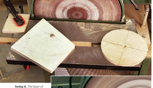
Swing it. The base of this jig pivots, allowing for adjustments to the diameter while in use. The short dowel registers in the hole centered in the back piece.
