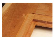
Rabbets. The view of the backside of the frame shows the shallow rabbet created during the first pass. The bit will be raised and the frame sent around again, until the final depth is achieved.
