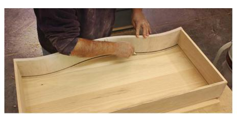
**Another transfer.** Drawer bottoms are milled to size and cut to slide into the  $^{1}/_{4}$ " grooves in the drawer boxes, but you need to shape the front edge to match the drawer front before you can slip them into place.
