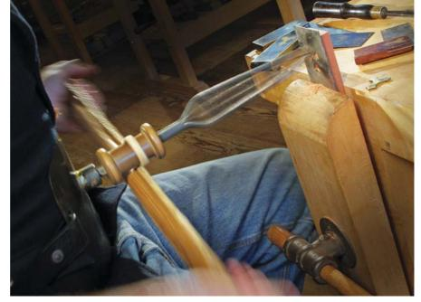
A rattling blur! The two prongs of the passer drill ride tightly within the walls of the template, routing out the pattern in seconds. To cut with square walls all around, the user keeps tilting the drill by shifting about in a circular manner - a process that looks as strange as it sounds!
