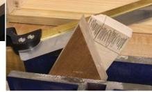
Miter aid. The bottom front must be trimmed flush to the case side and have a mitered outside corner. I use a scrap cut at 45° to help guide my saw for the miter cut.
