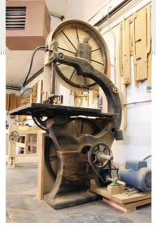
Massive iron. Tipping the scales at 1,275 pounds, this Jones Superior band saw has wooden wheels that Miller trued up using a router iig.
