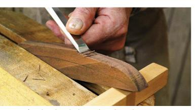
**Sharp tip.** A sharp chisel can work wonders on sharp curves to erase any sawblade marks or sanding scratches.
