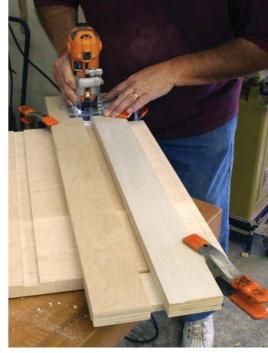
**Shop-made jig.** Make drawer runner dados easily and quickly with a simple jig built out of plywood.
