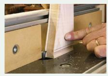
Finger-pressure tight. To set up the sliding dovetail cut, use drawer-blade offcuts. Set the height of the sliding dovetail before adjusting the width of your cut.
