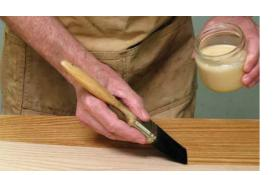
Brushing wiping varnish. Green paint thinner works well for making your own wiping varnish. Here, I'm brushing a homemade wiping varnish (half polyurethane and half green paint thinner) onto a panel. As explained in the November 2011 issue (#193), I can leave the wiping varnish as brushed. I can wipe it off. Or I can "dry brush" it
