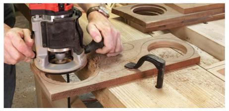
Orderly steps. Mill the rabbets before cutting the blanks to shape. That leaves material to support the router, and to clamp the work to the bench.
