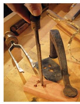
Connect the dots. Quick work with a gouge and you're ready to pop out the core between the foliated elements of the pattern. The shoulders on the business end of the passer drill stop the routing at the precise depth for the brass escutcheon.
