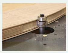
Stand-out detail. The bead detail is an important part of the drawer blade's edge profile. Router bits are a quick way to both cut the bead and raise it from the surface.
