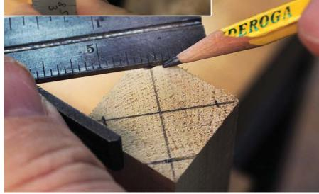
and eventually the fourth side of the blank. For this exercise we need to end up with a perfectly square blank that is 1" in width and thickness over its entire length-otherwise you won't end up with a perfect cylinder.
