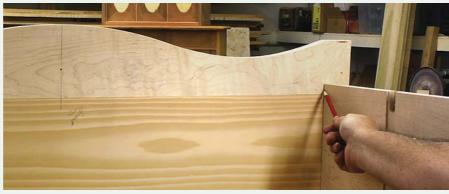
Sizing the drawer-blades. Align the centerline of the drawer blade with the centerline of the bottom. Mark the location where the blade meets the inside of the case sides.
