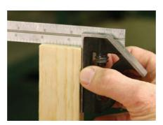
**Square is a must.** In any project, parts must be square or problems will arise. Use a combination square to check all perpendicular faces.
