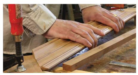
Taking sides. To index the moulding and hold it tight to the layout lines during glue-up, scraps are clamped at the layout lines.
