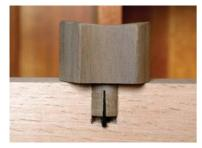
Foxed wedge. If your handle is attached with a dowel, you can wedge it in place by cutting a slot and then insert a wedge loosely in the slot. When the handle fully seats and the dowel bottoms out in the hole, the wedge will be pushed farther into the dowel and spread it for a tight fit.
