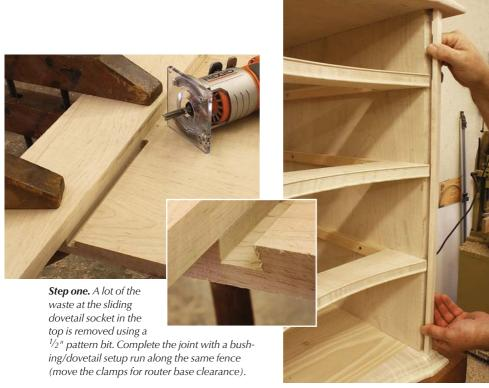
**Front face.** Fit then install the two front face pieces to the front edge of the case sides. Use glue and attach with 23-gauge pins.
