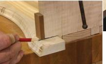
**Tricky layout.** A scrap simulates the  $\frac{3}{8}$ "-thick  $x^{3}/4$ "-wide front face that is added to the front edge of the sides to prepare for the vertical  $\frac{1}{8}$ " bead. Also note the notch for the bottom front.
