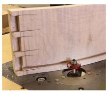
**Curved grooves?** A slot cutter in the router table is perfect for these cuts. Set the height of the cut at <sup>3</sup>/<sub>4</sub>" then run your grooves.
