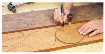
Crystal clear. A transparent pattern, made from <sup>3</sup>/8"-thick Lexan, makes it easy to adjust the position of the wood grain to the shape of the mirror.
