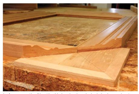
Lend me your ear. After all four sides of the frame have been glued to the face frame, each ear is treated as an individual frame.
