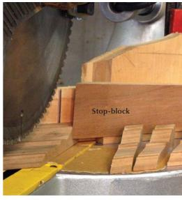
Mass miterer? A stop-block clamped to the fence allows identical parts to be cut with precision.
