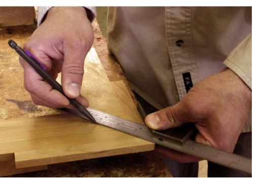
A simple layout. Two intersecting layout lines – one from the center to the outside corner, and another from inside corner to inside corner of each ear – are all that is required.
