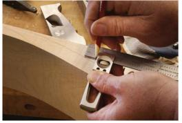
**Square shoulders.** Curved ends are not conducive to cutting dovetails. Add a straight section at the end to keep the corners at 90°.
