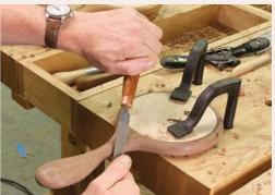
Rough to ready. A series of rasps removes the facets left by the spokeshave, eases the transitions between the curves and refines the shape.
