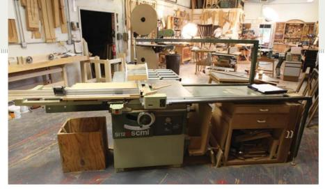
**Tweaked machinery.** An SCMI table saw is at the heart of Miller's shop. Note the shop-made blade guard (which he never removes) and the sliding fence, which Miller modified to satisfy himself.
