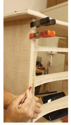
Fitting the beads. Miter one end of bead moulding stock, set it in place then mark the back of stock to easily determine the location of the second miter cut.
