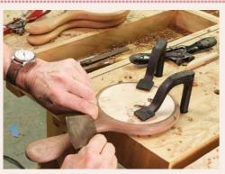
Like magic. A card scraper is ideal for following the rasp. It slices off the ridges left by the teeth of the rasp, leaving a smooth surface.
