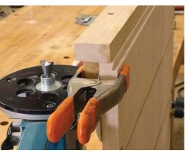
**Another simple jig.** To make my sliding dovetail jig, assemble a T shape then trim one arm so the resulting cut from the router setup leaves exactly  $\frac{3}{4}$ " to match the top's groove that will be cut later in the process.
