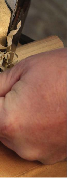
**16 sides.** This dowel blank started as a 1" square. With 16 sides planed, it's almost halfway to round.
