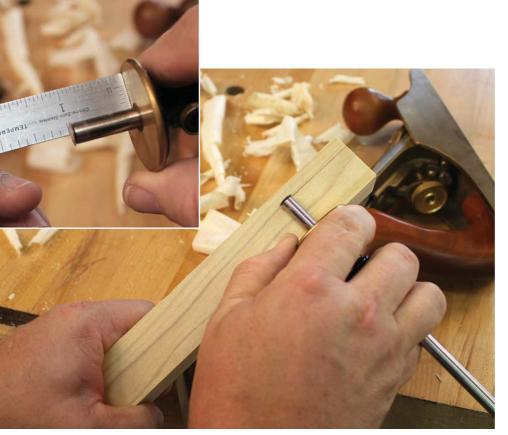
An inch square. To end up with a 1" dowel, you need a 1"-square blank. Set your marking gauge to 1" and, referencing off the two index surfaces, scribe that measurement on the other two faces of the blank. Plane down to those scribe lines. (If you have a great deal of waste to remove, saw the bulk of
