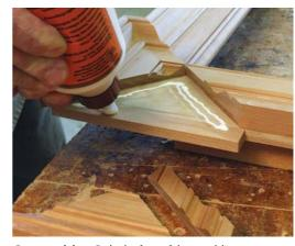
**Crossette icing.** Only the face of the moulding is glued. No adhesive is applied directly to the mitered edges – although some may creep up into the joint.
