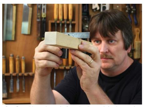
Adjacent flat. Handplane an adjacent surface flat, straight and square to the first. These two surfaces become your index surfaces from which the other two sides are squared and made parallel.
