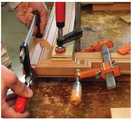
A nest of clamps. Clamps are added in a specific sequence to pull the pieces tight to one another.
