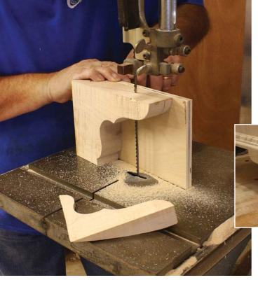
**Play it safe.** Without support of the work, your foot could be ripped from your hands as you make the band saw cut to shape the foot's front curve.
