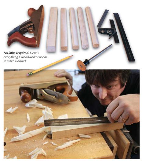
Reference surface. Handplane one side of the rough blank perfectly straight and flat. Use a straightedge to check it from side to side, over the length and from corner to corner to ensure your surface is perfectly flat.
