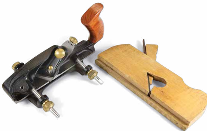
Complex animals. This wooden Russian standing rabbet plane is designed to cut a rabbet that's \frac{3}{8} " wide and that's it. The moving filer plane has an adjustable fence and a nicker. This one also has a skewed iron. Note I've removed the front knob of this plane—your off-hand should grasp the fence, not a knob.
