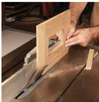
Bevel the underside. Run the frame on edge with the blade tilted to bevel the underside. Locate the bevel just below spline.
