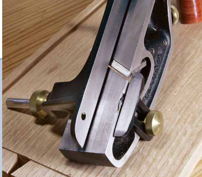
Skew for you? The skewed iron pulls the fence of this tool against the edge of the board, a handy feature.
