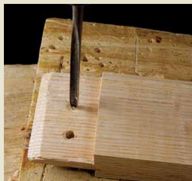
Fixed. In the end, all that will remain of these pins is a crescent-shaped fragment filling the errant hole.
