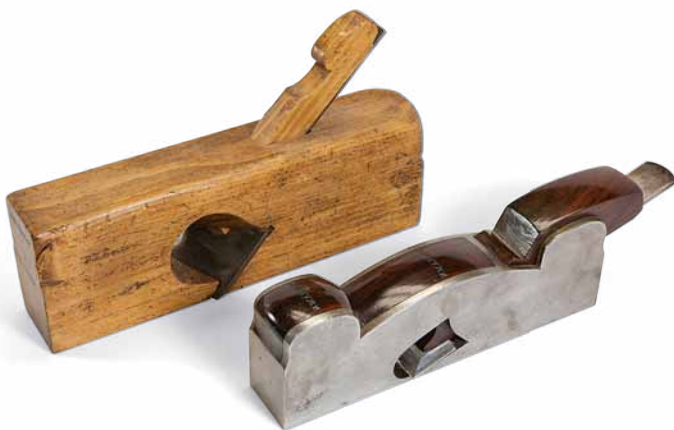
Rabbeting brothers. The simple rabbet lives up to its name—it is a block of wood, an iron and a wedge. This one is 1\frac{3}{4} " wide and its cutting angle is 45^\circ . The shoulder plane is like the simple rabbet but without the conical escapement. It also is made to tighter tolerances. It is 1\frac{1}{2} " wide and has a cutting angle of 47^\circ .
