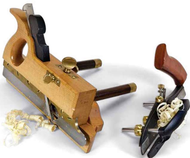
Metal & wood. Wooden plow planes throw the shavings onto your bench. Many modern metal plows throw the shavings into the fence's structure, where they can get in the way. I prefer tools that throw the shavings onto the bench.
