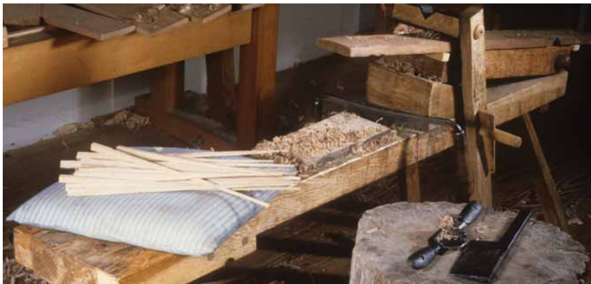
Alexander shaves the pins. Working long stock like this goes hand in hand with using the draw-knife and shaving horse. The extra length also lends itself to getting a long and gradual taper, the best form for these pins.
