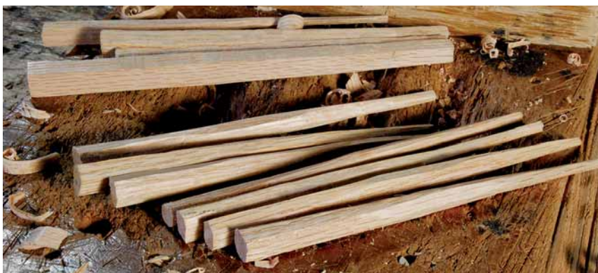
Facets. The pins we've found protruding inside stools and other joined works are usually faceted like the ones shown here. There's no need to make them perfectly round; driving them through the joint will burnish them to a degree.
