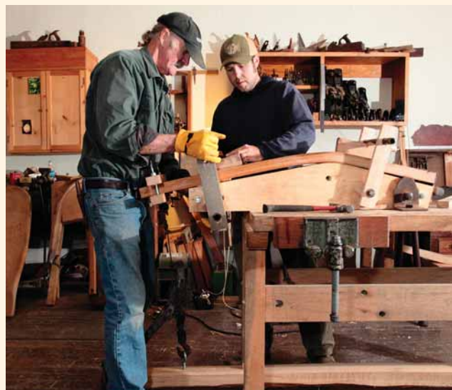
Hold on. A bracket and pipe holds the back to the form as it dries.
