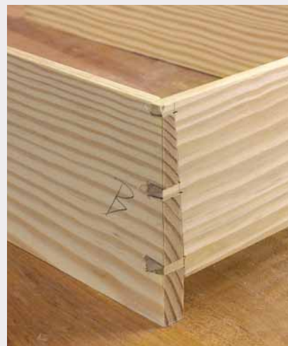
Up to the challenge? A through-dovetail – generally the easiest dovetail joint – becomes a bit more of a challenge when both parts are tapered.
