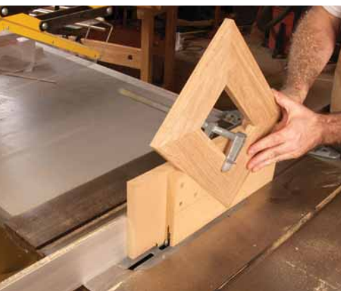
Spline the corners. When cutting the spline grooves, clamp the frame in the cradle jig with its top surface against the jig's face and locate the slots 1/8" in from the top surface.
