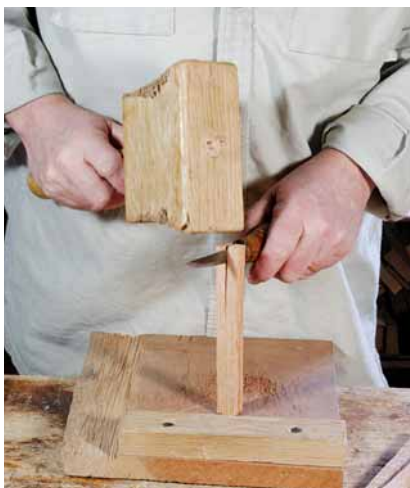
Follansbee rives. Riving principles apply here, just as on larger-scale stuff. Split in halves. Straight-grained stock is key. Never throw out any perfectly straight off-cuts, and keep a large supply on hand. The pins are the driest stock in the whole stool.
