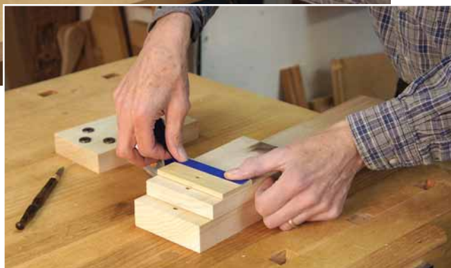
Drill with care. Position the parts to align the holes in all pieces. A leftover piece of spacer holds the work level.
