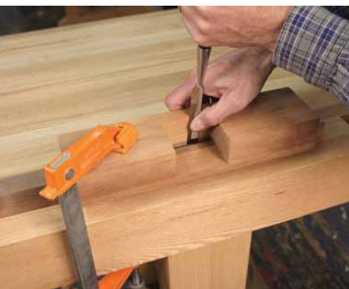
Crisp mortises. With this jig, you can pare all your mortise walls clean – hand cut or not.
