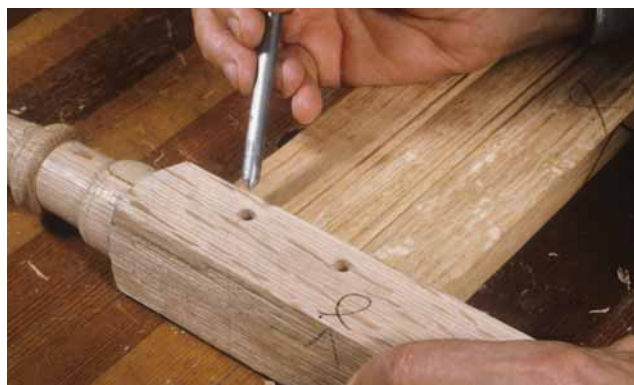
Alexander's marking technique. The centerpunch needs to fill the hole completely, so make one with material chosen to fit your boring tool. It makes a very clear depression on the tenon face.
