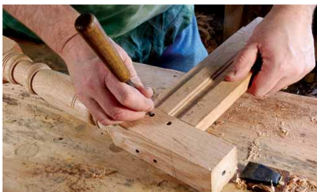
Follansbee's marking technique. The thinnest awl in the shop is best for marking your drawbore location. It can get right in against the circumference and transfer it accurately to the tenon's face.
