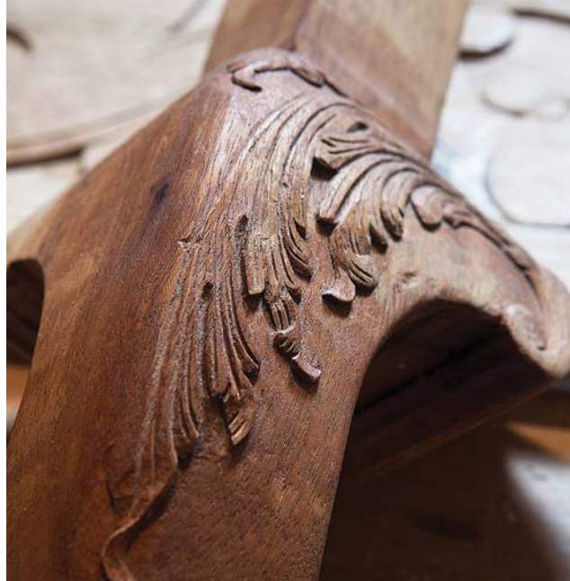
Detailed knee. Much of Mary's work involves ornamenting furniture built by others, such as this detail carving of an acanthus leaf on a cabriole leg.
