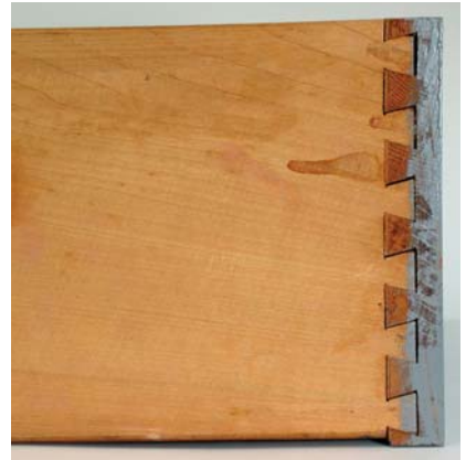
Machine-cut dovetail. A machine-cut dovetail establishes that the furniture wasn't made before 1895 when the machine that cuts these dovetails was invented.
