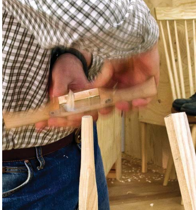
Reverse grip. A spokeshave can be used effectively with both a push and pull stroke. This is particularly useful when working on pieces such as spindles, where the grain often reverses. Notice the fingertip grip.
