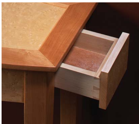
A hidden drawer. A false drawer front fits snugly between the legs so that when the drawer is closed you can't even tell it's there. A small cove routed on the underside of the drawer front allows you to pull it out from below.
