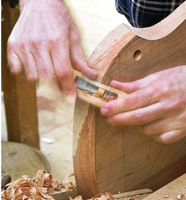
Thumb grip. The sole on this shave allows you to put your thumbs directly behind the blade for excellent tool control, without causing interference with the cuts.
