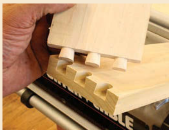
Half-blinds in a snap. Rounded tails fit snug into the rounded shoulders of the pins.
