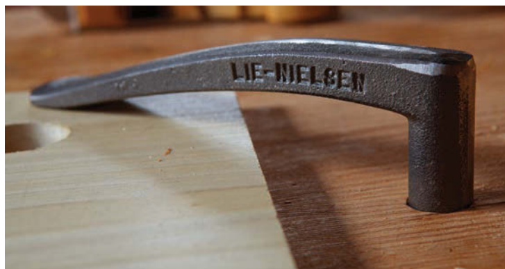
Lie-Nielsen Holdfast. The close-to-the-bench profile of this holdfast keeps it out of harm's way when you are pushing your planes around the benchtop.
