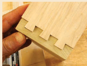
A tight fit. The assembled joint is mechanically sound and ready to assemble in a fraction of the time it would take to hand cut the joint.
