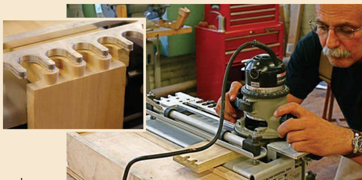
Simple dovetail jig. Easy to use, these jigs cut dovetails of a single size and rout both tails and pins at the same time.
