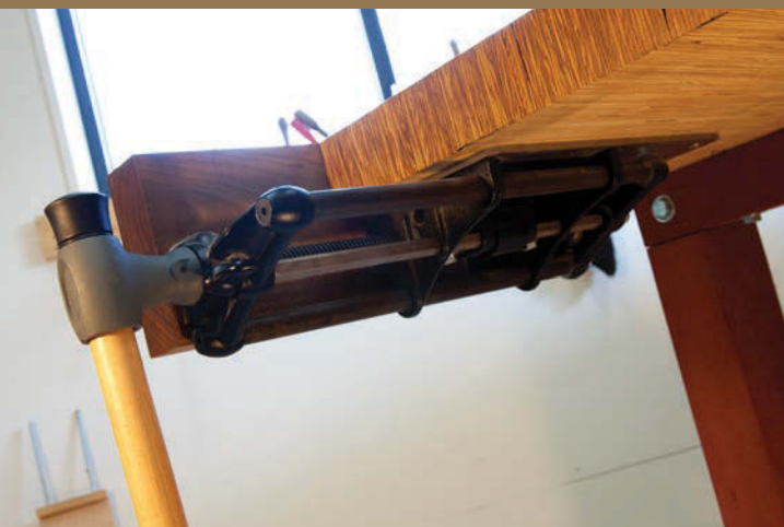
Veritas Quick-Release Sliding Tail Vise. This is the first tail vise I ever installed that doesn't sag. Add to that the fact that it offers quick-release and is simple to install and you'll know why it's one of my favorites.
