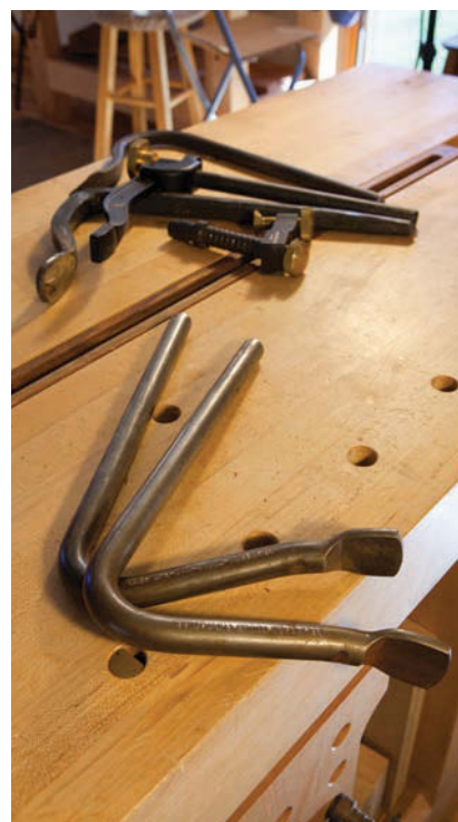
Gramercy Holdfast. This wire-formed holdfast (foreground) is the least-expensive effective holdfast on the market.
