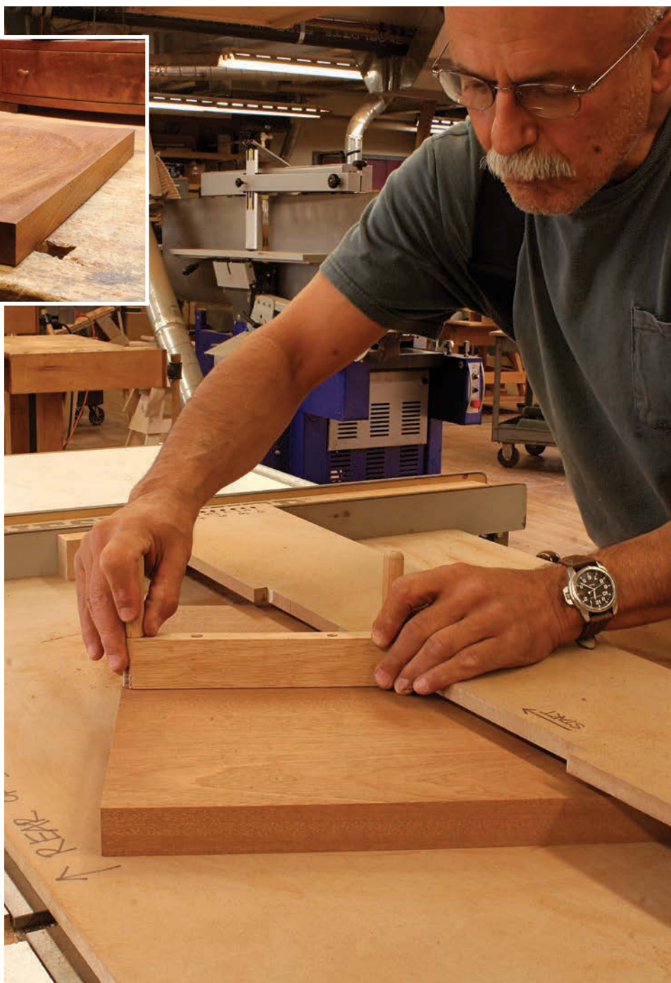
One big scoop. With a simple, shop-made jig, a table saw can make quick work of scooping a chair seat.
