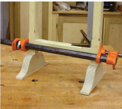
Check for racking. Because it's so easy to rack the small assembly, it's not good enough to clamp without checking for square.
