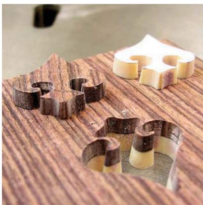
Inside passage. Here's the background (the wood) and waste from an interior cut
