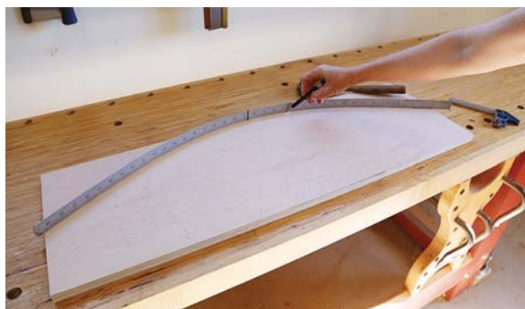
Patternmaker. After cutting \frac{1}{2} "-thick plywood to the overall length and width of the sides, I used a flexible rule held in place around three nails to draw a fair curve for my pattern.
