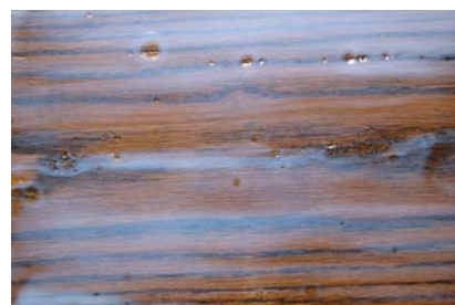
Not just a solvent-based problem. Fish eye can occur in water-based finishes, but emulsified fish-eye eliminators that mix well with these finishes aren’t widely available. So use a shellac sealer coat instead, or clean all the silicone off the surface before finishing.
