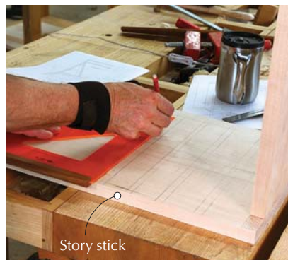
Plan meets reality. With the case dry-fit, dados for interior partitions are laid out from a story stick.
