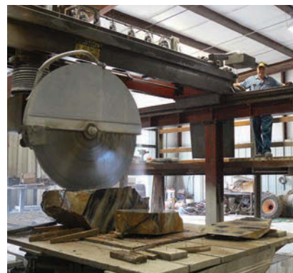
Now that's a saw. Large chunks of stone are cut down to a workable size on this 54"-diameter stone saw.
