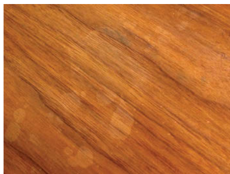
Watco watermarks. Watco Danish Oil claims better protection because the finish polymerizes "in" the wood. Here, I left puddles of water on three coats of dried Watco for just more than a minute. It's clear that resistance to water penetration is very minimal.
