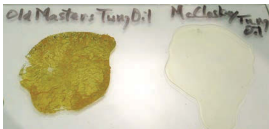
Two tung oils. Both of these products claim to be tung oil. Old Masters' (left) clearly is. McCloskey's (right) clearly isn't. It's varnish.
